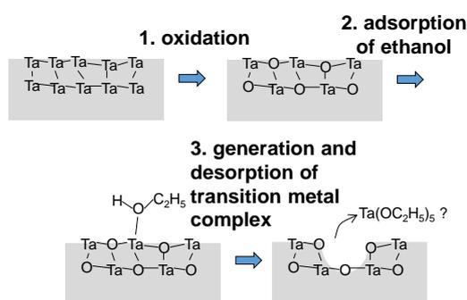
Fig. 3 Assumed mechanism of etching process.
