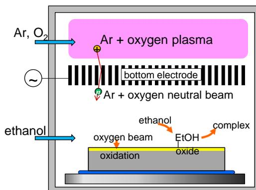
Fig. 2 Experimental setup using neutral beam to etch transition metals.
