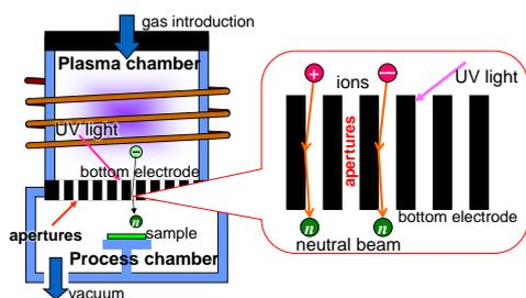
Fig. 1 Neutral beam apparatus.
