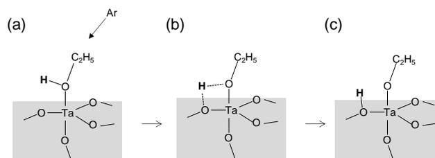
Fig. 5 Hydrogen movement reaction by argon bombardment.
