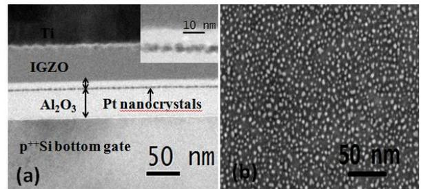
Fig. 2 (a) Cross-sectional TEM image of fabricated memory device and (b) SEM image of Pt nanocrystals.
