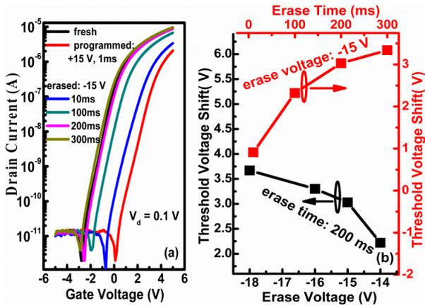
Fig.6 Erase characteristics of the programmed device as a function of erasing time and erasing voltage.
