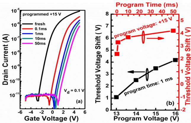
Fig. 5 Programming characteristics of the memory devices as a function of programming time and voltage, respectively.
