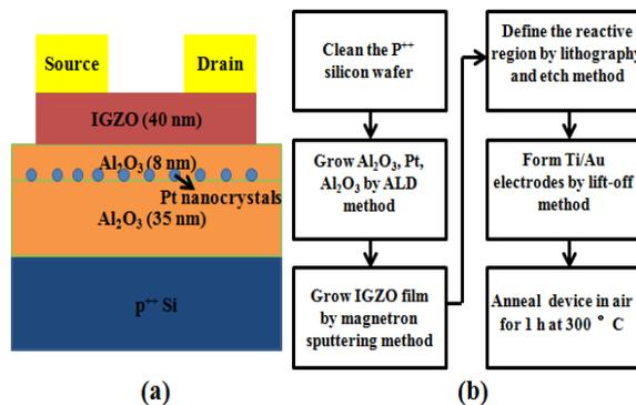
Fig. 1 (a) Schematic cross-sectional view and (b) process flow of the fabricated device.
