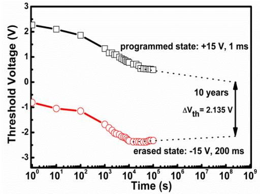
Fig. 7 Data retention characteristics of the memory at RT.
