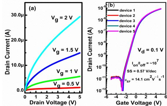
Fig. 3 The output (a) and transfer (b) characteristics of the fabricated TFT devices with Pt-NCs.
