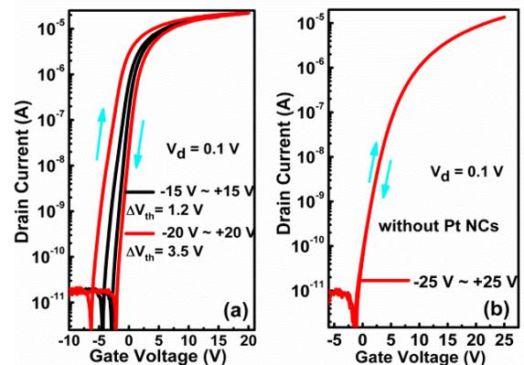
Fig. 4  $I_d$ - $V_g$  hysteresis behaviors of the TFT devices: (a) with Pt-nanocrystals; (b) without Pt-nanocrystals.
