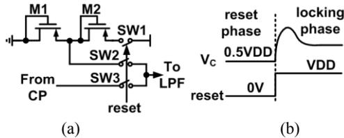
Fig. 2 (a) Schematic of the proposed start-up circuit. (b) Operation process of proposed SBPLL.
