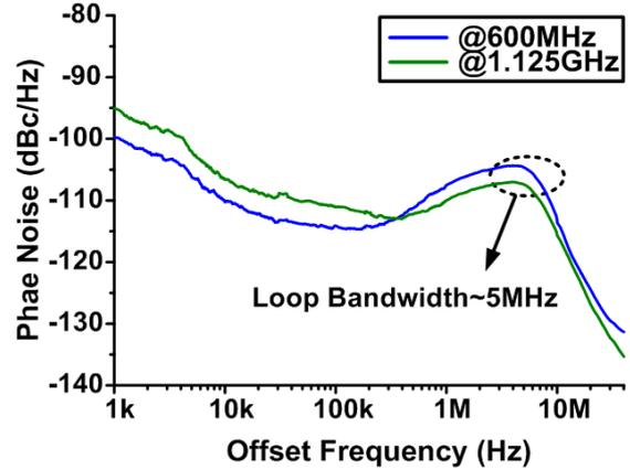
Fig. 4 Phase noise at 1.125GHz and 600MHz, respectively.
