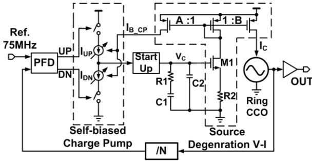
Fig. 1 Block diagram of the proposed SBPLL.
