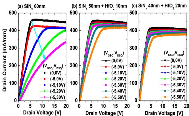
Fig. 4 Pulsed I-V characteristics of fabricated devices with different passivation layers (gate width =  $2 \times 50 \mu m$ ). Measurements for 500 ns pulse duration at  $V_{GS} = 0V$ .
