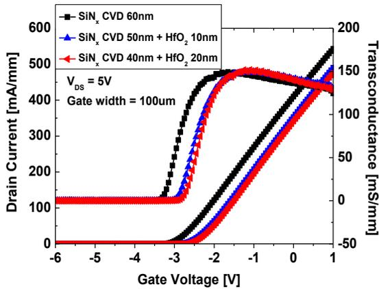
Fig. 2 Transfer characteristics of fabricated devices with different passivation layers at  $V_{DS} = 5V$ .
