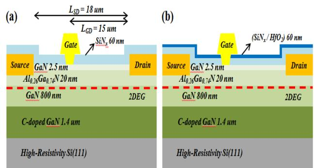
Fig. 1 Structures of fabricated devices (a) using only SiN<sub>x</sub> passivation layer and (b) using SiN<sub>x</sub> / HfO<sub>2</sub> dual passivation layer.
