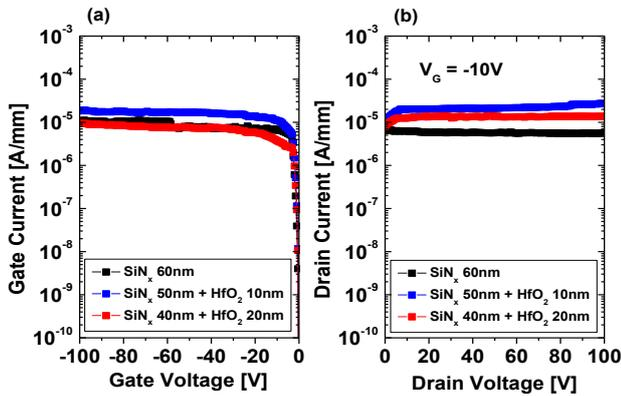
Fig. 3 (a) Gate reverse leakage currents and (b) Drain off-state leakage currents of the devices with three different passivation layers (gate width =  $100 \mu m$ ).
