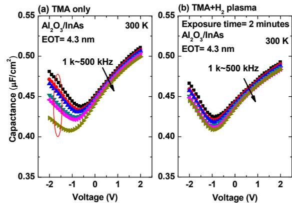
Fig.2 Room temperature multi-frequency C-V characteristics of Al<sub>2</sub>O<sub>3</sub>/InAs MOSCAPs with (a) TMA treatment only and (b) hydrogen plasma treatment prior to high-κ deposition
