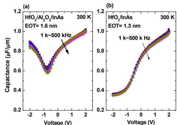
Fig.3 Room temperature multi-frequency C-V characteristics of (a) HfO<sub>2</sub>/Al<sub>2</sub>O<sub>3</sub>/InAs and (b) HfO<sub>2</sub>/InAs MOSCAPs with hydrogen plasma treatment prior to high-κ deposition
