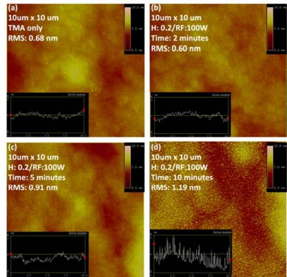
Fig.1 Atomic force microscopy of Al<sub>2</sub>O<sub>3</sub>/InAs surfaces treated by (a) TMA only, and hydrogen plasma for (b) 2 minutes, (c) 5 minutes, and (d) 10 minutes.
