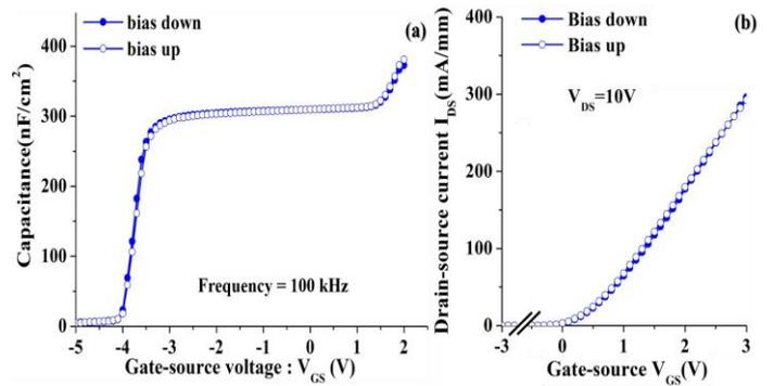
Fig. 4 (a) Hysteresis of capacitance-voltage curve. (b) Hysteresis of  $I_{\text{DS}}-V_{\text{GS}}$  curve of gate recessed MIS-HEMTs with  $\text{HfO}_2/\text{La}_2\text{O}_3$  stack gate insulator.
