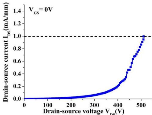
Fig. 3. The off-state breakdown characteristic of gate recessed MIS-HEMTs with  $\text{HfO}_2/\text{La}_2\text{O}_3$  stack gate insulator.
