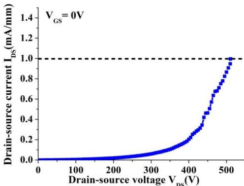
Fig. 3. The off-state breakdown characteristic of gate recessed MIS-HEMTs with  $\text{HfO}_2/\text{La}_2\text{O}_3$  stack gate insulator.
