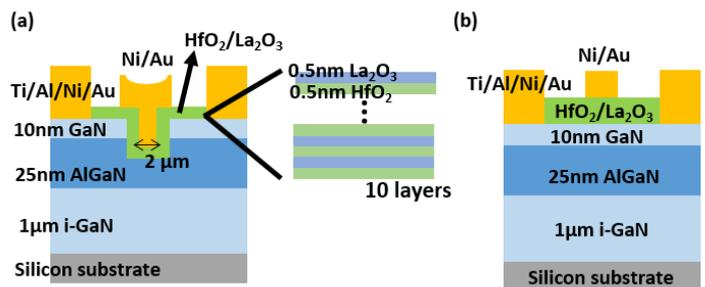
Fig. 1. (a) The structure of the device (b) The structure of the MOS capacitor.
