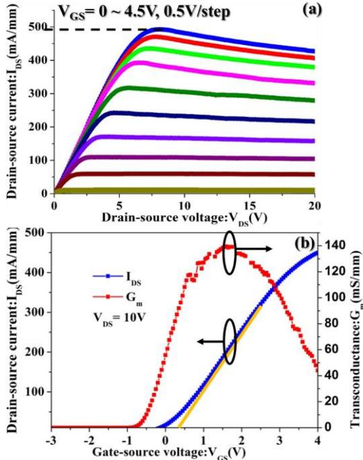
Fig. 2. (a)  $I_{\text{D}}-V_{\text{D}}$  characteristics (b)  $I_{\text{D}}/G_{\text{m}}-V_{\text{G}}$  characteristics of gate recessed MIS-HEMTs with  $\text{HfO}_2/\text{La}_2\text{O}_3$  stack gate insulator.
