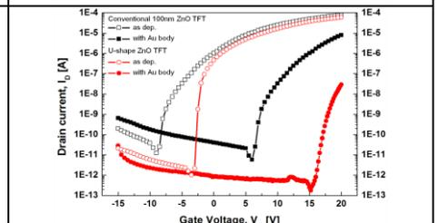
**Fig. 7.** Transfer characteristics of the fabricated ZnO TFTs with Au body metal contact: black symbols for conventional 100 nm ZnO TFTs and red symbols for U-shape ZnO TFTs. The solid symbols are for U-shape devices with Au body metal contact.
