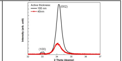
**Fig. 3.** XRD spectra of ZnO films according to the film thickness. The XRD peak at 34.1 represents the (002) ZnO crystal plane.
