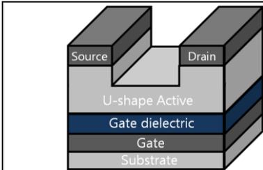
**Fig. 1.** Cross section of the suggested bottom gated U-shape ZnO TFT which is proposed to modulate  $V_{th}$  based on the thickness control of active layer without contact resistance deterioration. The channel width/length (W/L) is 2000/500  $\mu\text{m}$ .
