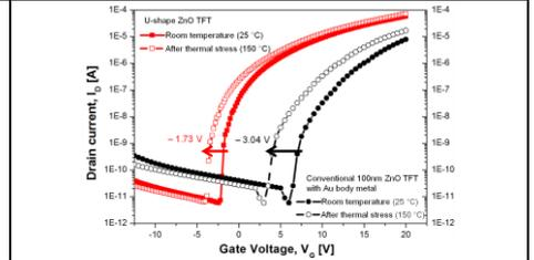
**Fig. 6.** Transfer characteristics of U-shape structure and conventional 100 nm ZnO with Au body metal TFT. Dash lines are thermal stress after 30 minutes at 150 °C.
