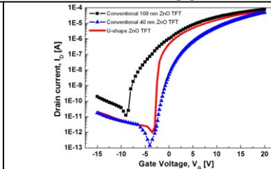
**Fig. 2.** Transfer characteristics of the fabricated ZnO TFTs as a function of the device structures: black square symbol is for the conventional TFT with 100 nm ZnO thickness, blue symbol for 40 nm ZnO and red line for U-shape. Here,  $V_{DS}$  is 20 V.
