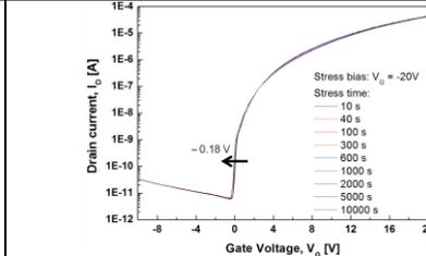
**Fig. 5.** Transfer characteristics of the U-shape ZnO TFTs with gate bias stress of -20 V which shows that the transfer curve shifts only -0.18 V after stress during  $10^4$  sec in the U-shape ZnO TFT. The applied  $V_{DS}$  is 20 V.
