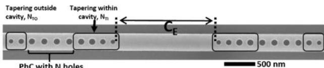
**Fig. 1** SEM image of a long/extended cavity with the cavity length,  $C_E$
