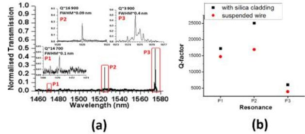
**Fig. 3:** (a) Measurement result for ultra-high Q suspended wire with extended cavity of  $C_E=4 \mu\text{m}$  (b) Comparison of the resonance Q-factor value with the suspended wire waveguide
