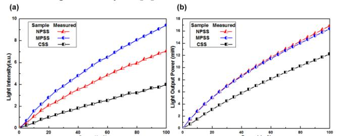
Fig. 5 (a) L-I characteristics of unpackaged and (b) packaged InGaN-based LEDs having the CSS, NPSS and MPSS.
