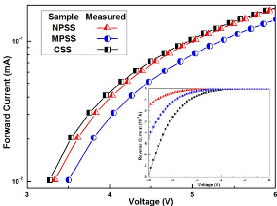
Fig. 4 Forward I-V characteristics and reversed I-V characteristics of InGaN-based LEDs having the CSS, NPSS and MPSS.
