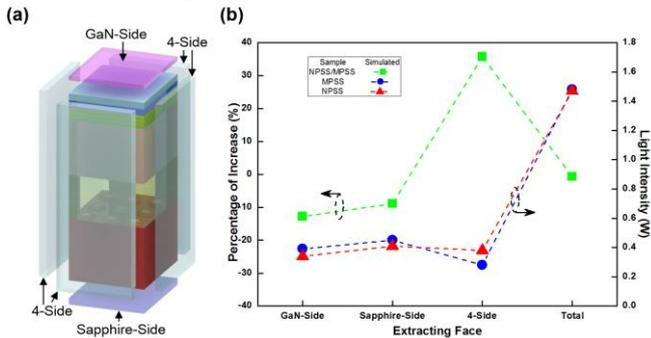
Fig. 3 (a) Schematic diagram of different receiver positions considered in the simulation. (b) Light Intensity and percentage of increase of InGaN-based LEDs grown on the NPSS and MPSS detected at different detector.
