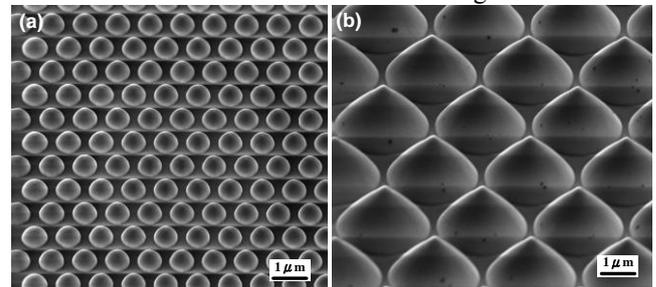
Fig. 1 The 52 degree tilted SEM images of (a) NPSS and (b) MPSS.
