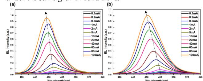
Fig. 2 Blue shifts phenomenon of the InGaN-based LEDs having the (a) NPSS and (b) MPSS.
