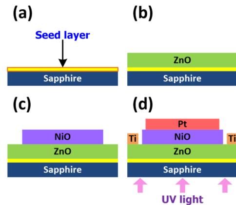
Fig. 1 Schematics of the fabrication process of the p-NiO/film-ZnO HJ.
