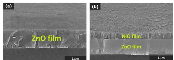
Fig. 2 SEM images of (a) HTG-ZnO film (900 nm) and (b) after NiO layer (300 nm) deposition.
