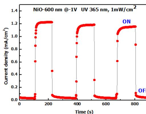
Fig. 6 Transient response of photocurrent density.
