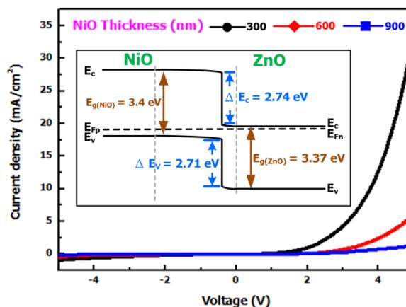
Fig. 5 The J-V curves of the p-NiO/HTG-ZnO films HJs in dark. The inset shows the energy band diagram of the p-NiO/n-ZnO HJ under thermal equilibrium.
