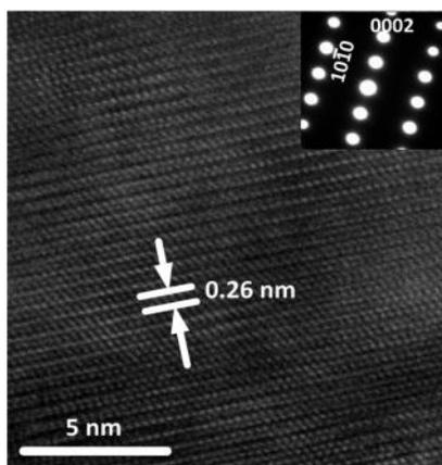
Fig. 4 TEM image and the corresponding SAED patterns of single-crystalline ZnO film.
