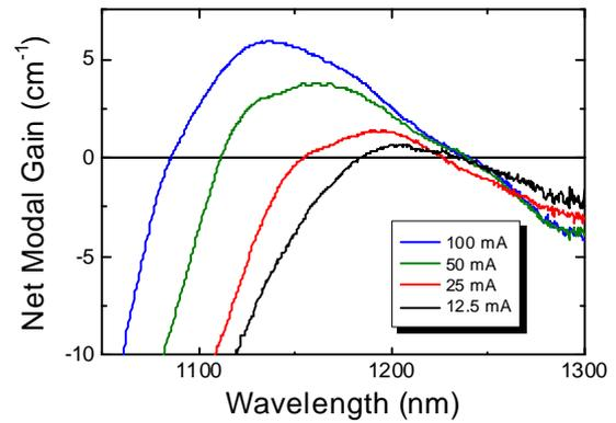
Fig. 3 Net modal gain spectra of the QD-SLD under various injection currents.
