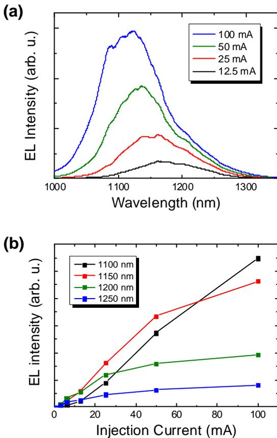
Fig. 2 (a) EL spectra obtained from the fabricated chip under various injection currents through the contact nearest to the edge. (b) EL intensity plotted for each wavelength as a function of injection current.
