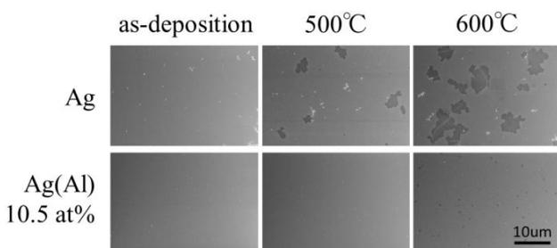
Fig. 3 SEM images of DMD films with pure Ag and with 10.5% Al-doped Ag layer at different annealing temperatures.
