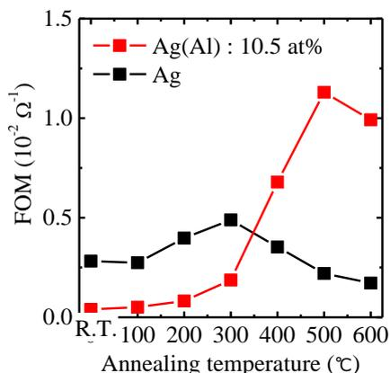
Fig. 4 Figure of merit of DMD films with pure Ag and with 10.5% Al-doped Ag layer as a function of annealing temperatures.
