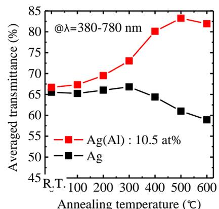
Fig. 2 Annealing temperature dependency of the average transmittance  $T_{\text{AVE}}$  in visible region (380-780 nm).
