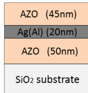
Fig. 1 Schematic diagram of AZO/Ag(Al)/AZO-DMD.
