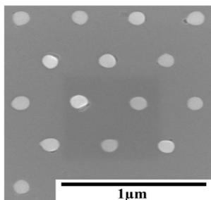
Fig. 4 FESEM image of selective-area Ga droplet deposition on top of as-grown n-GaAs nanostub buffer layer on Si(100)
