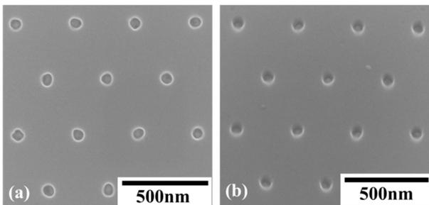
Fig. 3 FESEM (a) plan view and (b) tilted view images of selectively grown sub-100nm n-GaAs nanostub thin buffer layer on SiO<sub>2</sub>-patterned Si(100)
