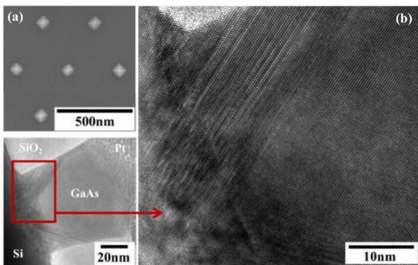
Fig. 2 (a) FESEM and (b) HRXTEM images of 50nm n-GaAs nanostubs on Si(100)
