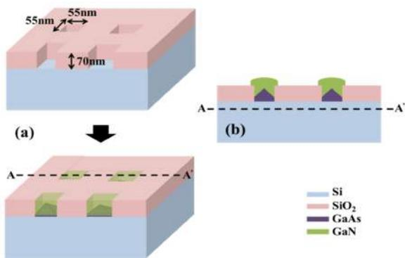
Fig. 1 Schematic diagram of (a) selective-area epitaxy of sub-100nm n-GaN/GaAs nanostubs on Si(100) and (b) cross-section cut along A-A'
