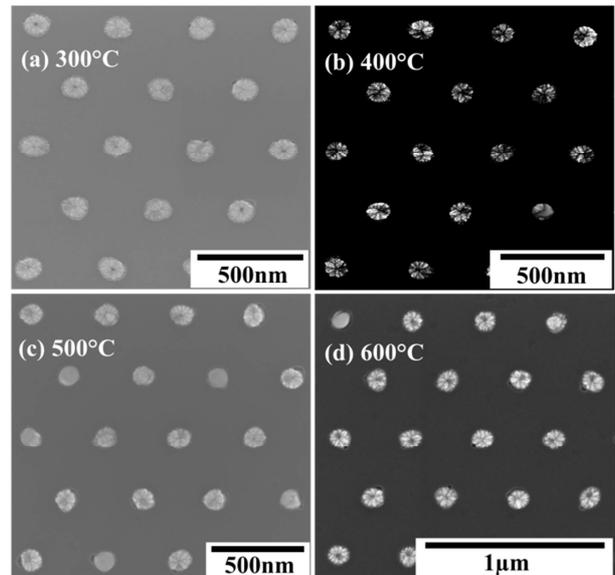
Fig. 5 FESEM images of selectively grown Ga droplet nitridation at (a) 300°C (b) 400°C (c) 500°C and (d) 600°C
