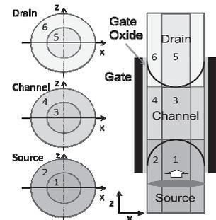
Fig.8 The pillar is divided into six regions for evaluating the path of electron in the channel
