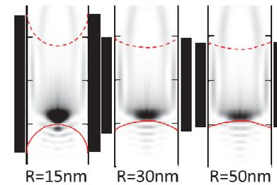
Fig.4 Snapshot of electron density at 0.1ps for various radius of curvature.
