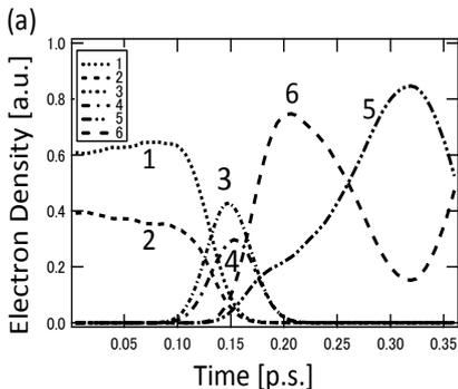
Fig.9 Time dependence of electron density in each pillar region (see Fig.8). The height in the channel is (a) 100meV, (b) 200meV.
