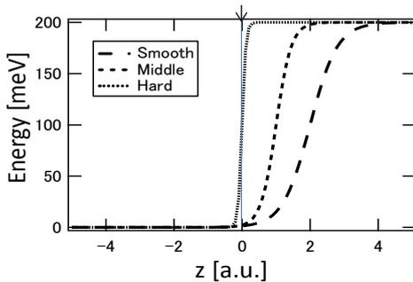
Fig.6 The potential profiles for the source-channel direction
