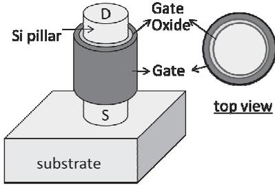
Fig.1 Schema of vertical body channel (VBC) MOSFET, where the whole body is working as the channel [5]
