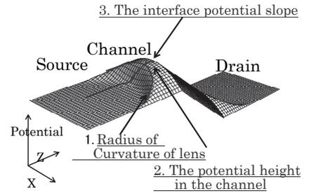
Fig.3 Lens Potential Parameters
