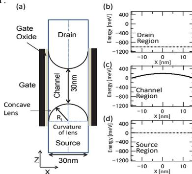
Fig.2 (a) The structure of VBC-MOSFET with lens. (b)-(d) show the potential profile of x direction in the source, the channel, and the drain, respectively.
