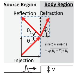
Fig.5 The reflection manner of electron at the potential interface.
