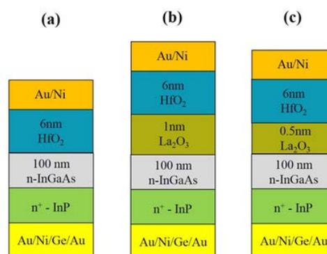
Fig. 1 Schematic illustration of fabricated (a)  $\text{HfO}_2(6\text{nm})$  (b)  $\text{HfO}_2(6\text{nm})/\text{La}_2\text{O}_3(1\text{nm})$  (c)  $\text{HfO}_2(6\text{nm})/\text{La}_2\text{O}_3(0.5\text{nm})$  MOS capacitors
