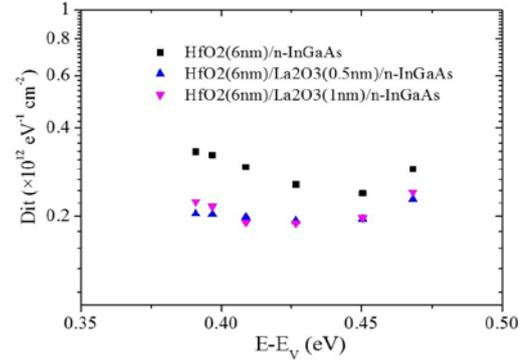
Fig. 3 Interface trap density distribution of the sample extracted by conduction method at 77K.
