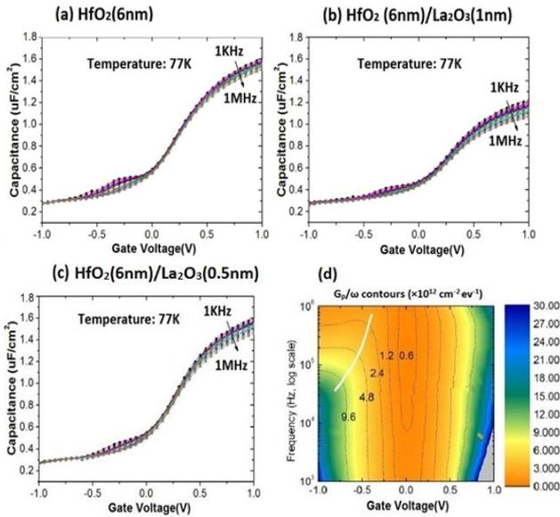
Fig. 2. Multi frequency C-V curve at 77K of the (a)  $\text{HfO}_2(6\text{nm})$  (b)  $\text{HfO}_2(6\text{nm})/\text{La}_2\text{O}_3(1\text{nm})$  (c)  $\text{HfO}_2(6\text{nm})/\text{La}_2\text{O}_3(0.5\text{nm})$  MOS capacitors after PDA at  $450^\circ\text{C}$  in  $\text{N}_2$  for 5 minutes and (d) Normalized parallel conductance contour map for the  $\text{HfO}_2(6\text{nm})/\text{La}_2\text{O}_3(0.5\text{nm})$  MOS capacitor
