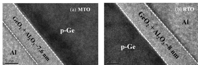
Fig. 3 TEM images of Al/Al<sub>2</sub>O<sub>3</sub>/GeO<sub>2</sub>/p-Ge gate stack with GeO<sub>2</sub> grown by (a) MTO (b) RTO.
