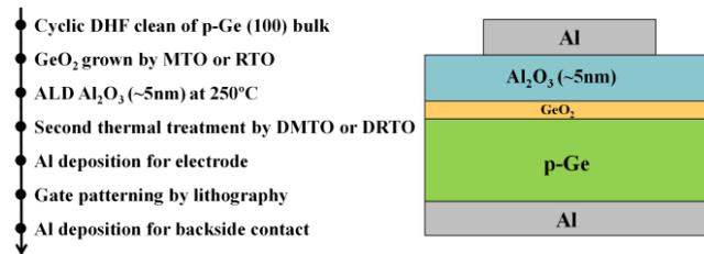
Fig. 2 Process flow and schematic structure of Al/Al<sub>2</sub>O<sub>3</sub>/GeO<sub>2</sub>/p-Ge MOSCaps.
