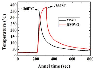
Fig. 1 Temperature (°C) versus anneal time for MTO and DMTO.
