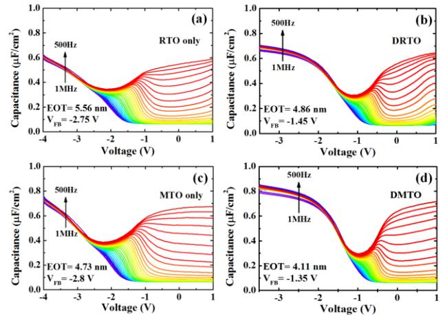
Fig. 4 C-V characteristics of Al/Al<sub>2</sub>O<sub>3</sub>/GeO<sub>2</sub>/p-Ge MOSCaps with GeO<sub>2</sub> grown by (a) RTO only (b) DRTO (c) MTO only (d) DMTO respectively.
