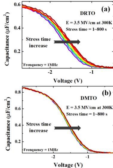
Fig. 6 C-V characteristics of Al/Al<sub>2</sub>O<sub>3</sub>/GeO<sub>2</sub>/p-Ge MOSCaps under constant field FN stress for (a) DRTO and (b) DMTO cases.
