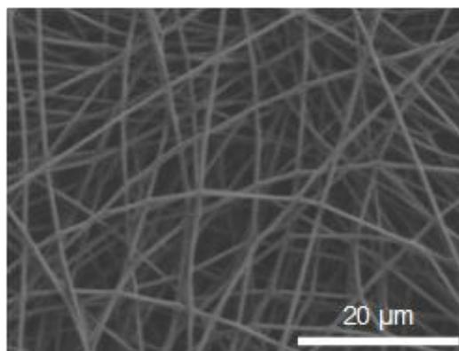
Figure 1. FE-SEM image of the surface of an electrospun PDLLA fibrous film.
