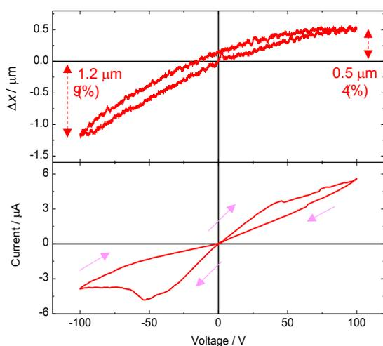
Figure 2. Displacement of the surface of an electrospun PLA-fiber film and the displacement current flowing in the film versus the applied voltage—a triangular wave with a scan rate of 6 V/s and amplitudes of  $\pm 100$  V<sub>pp</sub>.
