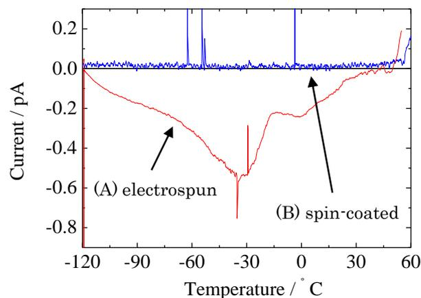
Figure 3. TSC spectra for (A) an electrospun film and (B) a spin-coated film of PDLLA without a poling treatment. The scanning temperature range was in the range of  $-120$ – $60$  °C with a heating rate of  $10$  °C/min.
