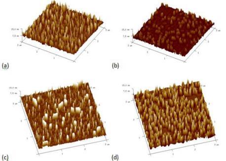
Fig. 2 AFM of high-k BaSrTiO<sub>3</sub> surface on single crystalline silicon after RTA at different temperatures (a) RTA 600°C in N<sub>2</sub> R<sub>rms</sub>=1.312(nm) (b) RTA 700°C in N<sub>2</sub> R<sub>rms</sub>=0.898(nm) (c) RTA 600°C in O<sub>2</sub> R<sub>rms</sub>=2.254(nm) (d) RTA 700°C in O<sub>2</sub> R<sub>rms</sub>=1.733(nm)
