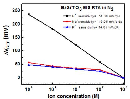
Fig. 6 The different ion sensitivity of BaSrTiO<sub>3</sub> sensing membrane annealed at 600°C in N<sub>2</sub> ambient
