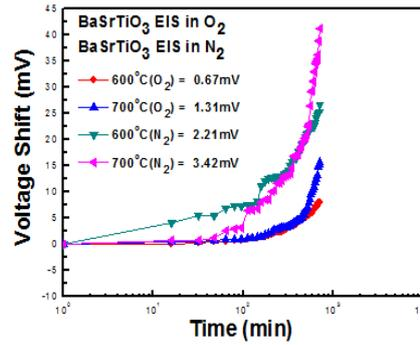
Fig. 5 Drift voltage of BaSrTiO<sub>3</sub> sensing membrane annealed with various RTA temperatures in N<sub>2</sub> and O<sub>2</sub> ambient, then dipped in pH 7 buffer solution for 12 hours
