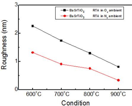
Fig. 2 (e) The comparison of AFM analysis for BaSrTiO<sub>3</sub> in different gas (N<sub>2</sub> or O<sub>2</sub>)
