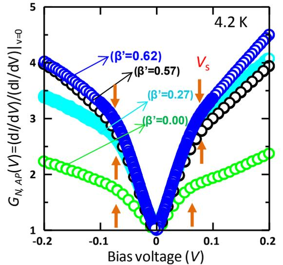
Fig. 2. Normalized  $dI/dV$  vs.  $V$  characteristics for AP in a small bias voltage region of up to  $\pm 0.20$  V for CMFS MTJs having various  $\beta'$  in  $\text{Co}_2\text{Mn}_{0.73}\text{Fe}_{\beta'}\text{Si}_{0.84}$  electrodes ( $\beta' = 0.0, 0.27, 0.57$  and  $0.62$ ).
