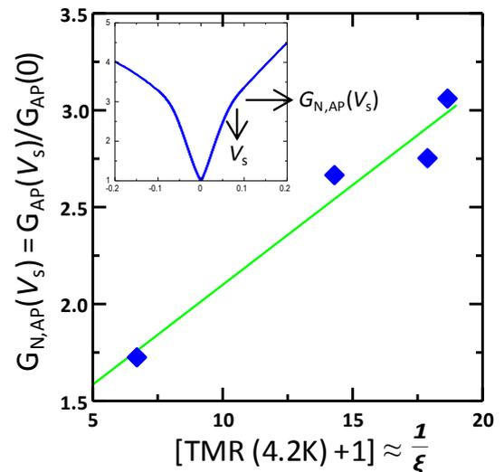
Fig. 3. Normalized  $G (= dI/dV)$  values at  $V = V_s (= 70$  mV) for CMFS MTJs as a function of  $(\text{TMR}(4.2\text{K}) + 1)$ .
