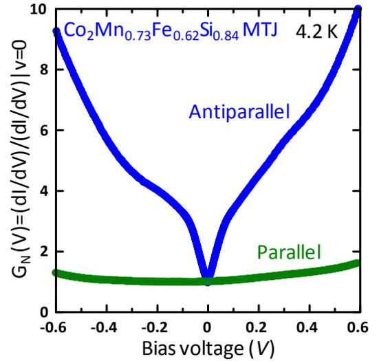
Fig. 1. Normalized  $dI/dV (= G)$  vs.  $V$  characteristics for P and AP of a CMFS MTJ with  $\text{Co}_2\text{Mn}_{0.73}\text{Fe}_{0.62}\text{Si}_{0.84}$  electrodes that exhibited a TMR ratio of 1765% at 4.2K.
