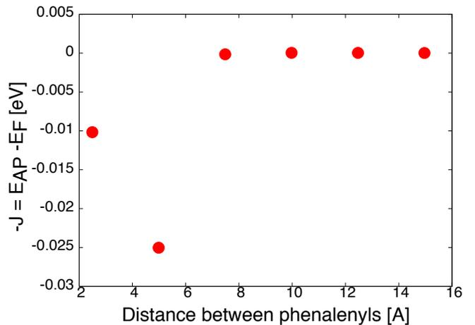
Fig. 4 The spin-spin interaction  $J$  between two graphene flakes as a function of the interflake spacing.
