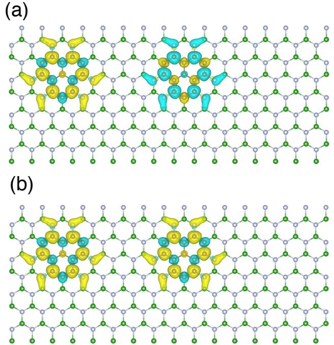
Fig. 3 Ipsurfaces of spin densities of graphene flakes embedded into h-BN with the flake-flake spacing of 1 nm in (a) an antiparallel and (b) parallel spin arrangements. Colors denote the sign of spin components. Green, white, and brown circles denote B, N, and C atoms, respectively.
