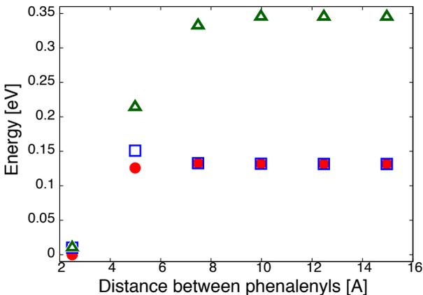
Fig. 2 Calculated total energy of graphene flakes embedded into h-BN sheet as a function of distance between flakes. Energies are measured from the flakes with  $d = 0.25$  nm in antiparallel state.
