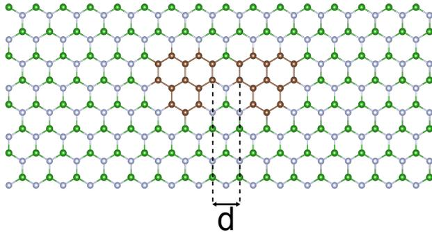
Fig. 1 Structural model of graphene flakes embedded into a h-BN sheet. Green, white, and brown circles denote B, N, and C atoms, respectively.
