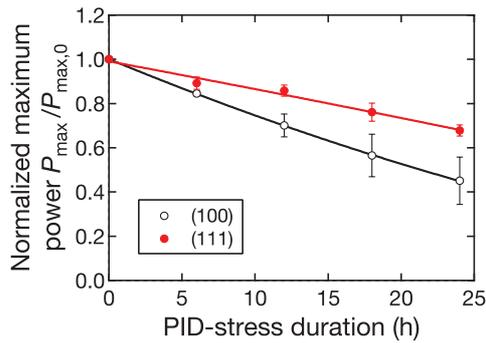
Fig. 1. Dependence of  $P_{\max}/P_{\max,0}$  of the modules with (100)- and (111)-oriented cells on PID-stress duration. Each data point shows the mean value for three modules, and each error bar corresponds to the standard error of the mean.
