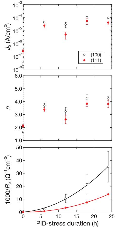
Fig. 2. Dependence of  $J_0$ ,  $n$ , and  $1000/R_p$  of the modules with (100)- and (111)-oriented cells on PID-stress duration. Each data point shows the mean value for three modules, and each error bar corresponds to the standard error of the mean.
