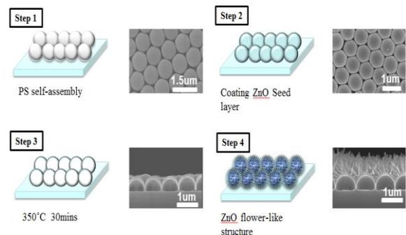
Fig. 1 Schematic process for fabricating the flower-like ZnO on conductive glass substrate
