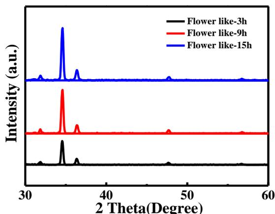
Fig. 3 X-ray diffraction patterns of flower-like pattern
