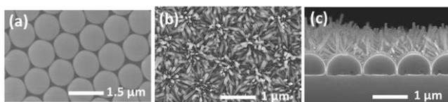
Fig. 2 SEM images of the flower-like ZnO pattern on silicon substrate
