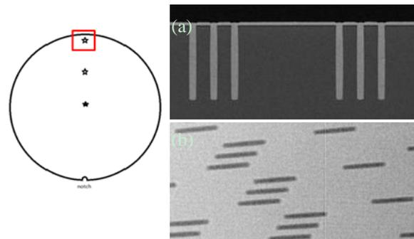
Fig.4 Cu plating results of the edge of 300mm wafer: SEM cross-section micrograph (a) and X-Ray image(b).
