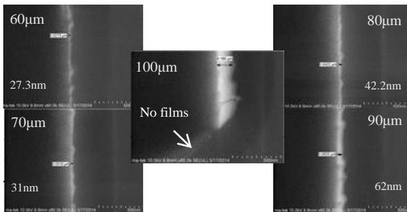
Fig.3 SEM micrographs of the process with high bias power corresponding to the area of 60μm to bottom corner.
