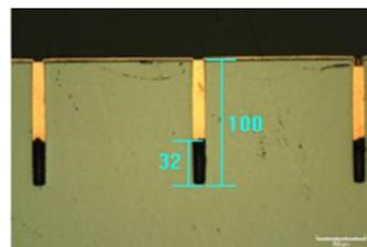
Fig. 1 The result of electroplating of 10x100 $\mu\text{m}$  TSVs with baseline PVD process.
