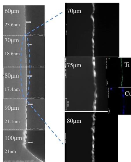
Fig. 2 SEM micrographs of the baseline process from the area of 60 $\mu\text{m}$  to bottom corner (left column of graphs), TEM micrographs of weakest area of 70 $\mu\text{m}$  to 80 $\mu\text{m}$ (right column of graphs) and EDX mapping of the position around 75 $\mu\text{m}$ (the right inserts).
