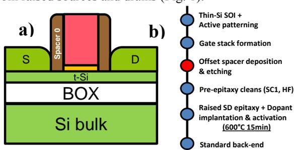
Fig. 1: a) MOSFET on planar FDSOI after raised source/drain epitaxy step; b) Simplified process flow
