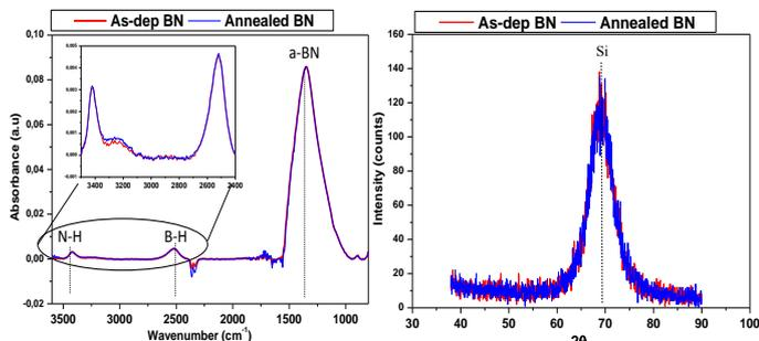
Fig. 3: Transmission FTIR (left) and XRD (right) spectra for as-deposited and annealed (600°C/15min) BN film.
