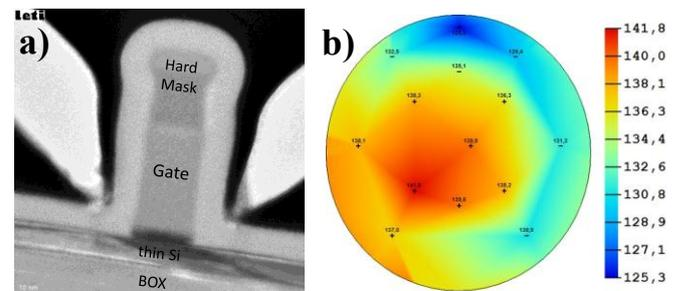
Fig. 4: a) TEM picture after BN deposition; b) thickness uniformity measured by ellipsometry.
