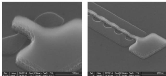
Fig. 2: SEM pictures of 500°C ALD  $\text{SiN}_x$  after plasma etching
