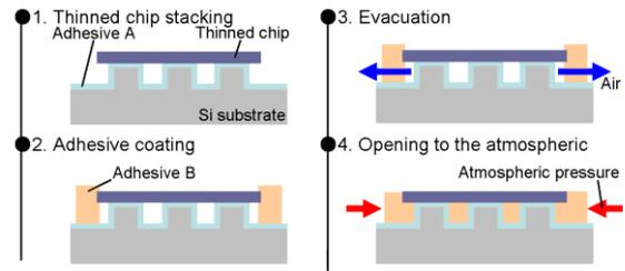
Fig. 4. Process flow of the test structure with Si microbumps.
