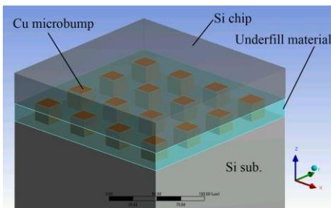
Fig. 2. Simulation model for analysis of local bending stress induced by the CTE mismatch and heat generation.
