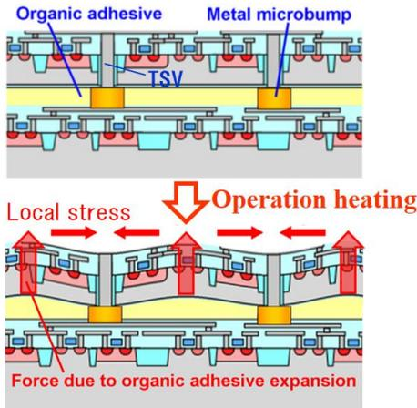
Fig. 1. Schematic cross-section of 3D IC expressing local stress due to adhesive expansion induced by heat generation in circuit operation and the CTE mismatch between organic adhesive and metal microbumps.
