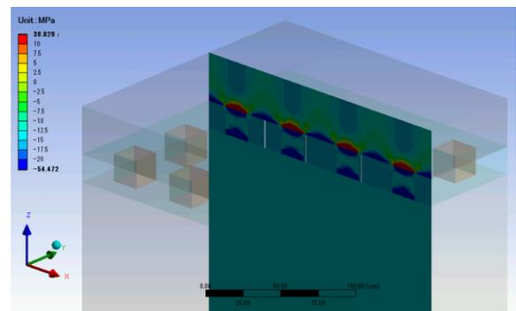
Fig. 5. Simulation result of normal stress on X direction at temperature changed from 23°C to 50°C.
