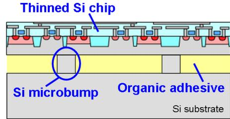
Fig. 3. Schematic drawing of the test structure to evaluate the effect of local bending stress due to organic adhesive expansion.
