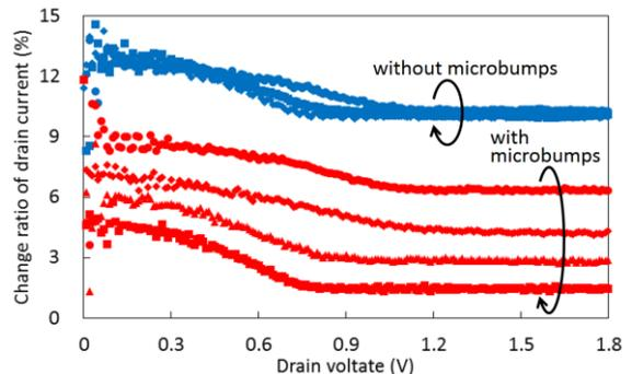
Fig. 6. Effect of local bending stress on drain current of pMOSFET fabricated in thin IC chip from 23°C to 50°C with and without Si microbumps.
