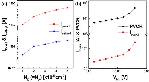
Fig. 3 (a) peak1 and valley1 currents according to doping concentration of  $pn$  tunnel diode (b) peak2 currents and 2<sup>nd</sup> PVCGR according to transition voltage ( $V_{\text{ML}}$  @  $V_G = V_{\text{DD}}/4$ ) of STI.
