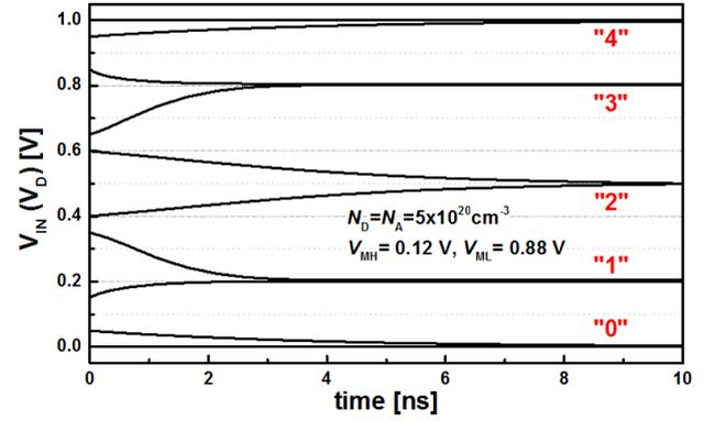
Fig. 4 Transient simulation results of the latch circuit. Initial states of  $V_{\text{IN}}$  with variation of  $\pm 100$  mV are converged to 5-states.
