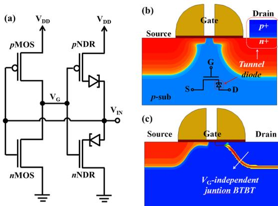
Fig. 1 (a) 5-state latch circuit composed with CMOS STI ( $n$ MOS and  $p$ MOS),  $n$ -type NDR ( $n$ NDR), and  $p$ -type NDR ( $p$ NDR) (b) 2-D cross sectional view and circuit symbol of  $n$ NDR [4] (c) 2-D cross section view and band-to-band generation view of  $n$ MOS for STI [5].
