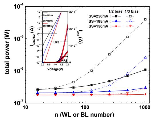
Fig. 1 Total power consumption according to the array size, SS of the selector, and bias schemes at  $V_{dd}=1.5V$ . (Inset graph: I-V characteristics of 1S and 1S+1R)
