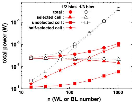
Fig. 3 Power consumption with (a) 1/2 and (b) 1/3 bias schemes at each region; selected cell, half selected cells, unselected cells. Selector SS =250mV,  $V_{dd}$ =1.5V.
