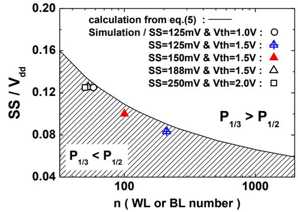
Fig. 4  $SS/V_{dd}$  with various SS and  $V_{th}$  of selector. The line represents the calculation result from Equation (5).
