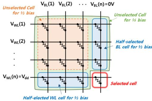
Fig. 2 Illustration of an  $n \times n$  crossbar array.
