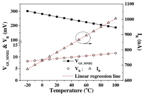
Fig. 2 Simulated temperature characteristics of  $V_{GS\_MND2}$ ,  $V_R$ , and  $I_R$  for bandgap temperature sensor using an off-chip ideal resistor.
