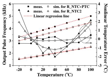
Fig. 4 Simulated and measured pulse frequencies against temperature, its linear regression line and nonlinear temperature error.
