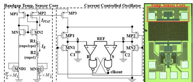
Fig. 1 The circuit schematic and chip photograph of the proposed temperature sensor with pulse output.
