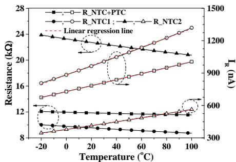
Fig. 3 Simulated temperature characteristics of resistance and  $I_R$  for bandgap temperature sensors using on-chip R\_NTC+PTC, R\_NTC1, and R\_NTC2, respectively.
