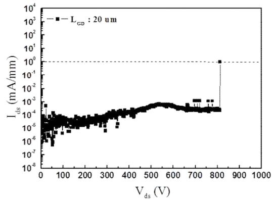
Fig. 2 Breakdown voltage of GaN HEMT
