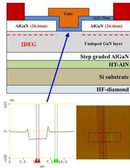
Fig. 1 Structure of GaN HEMT and profile of recessed gate
