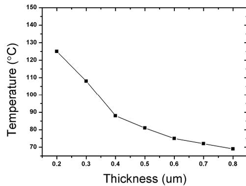
Fig. 3 Temperature of GaN power device during the high power operation vs thickness of diamond thin film as heat sink
