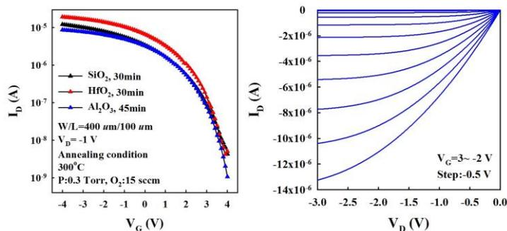
Fig. 6. (a) Transfer characteristics of SnO TFTs with various gate dielectrics and experienced sufficiently long annealing treatments. (b) Output characteristics of a SnO TFT with a SiO<sub>2</sub> gate dielectric.
