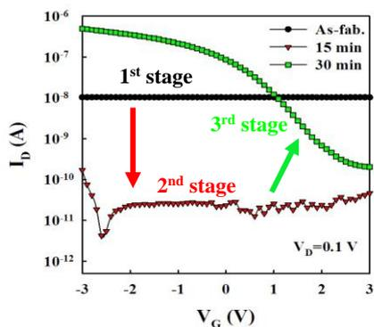
Fig. 2. Evolution of transfer characteristics with increasing CA time for a TFT with a SiO<sub>2</sub> gate oxide.
