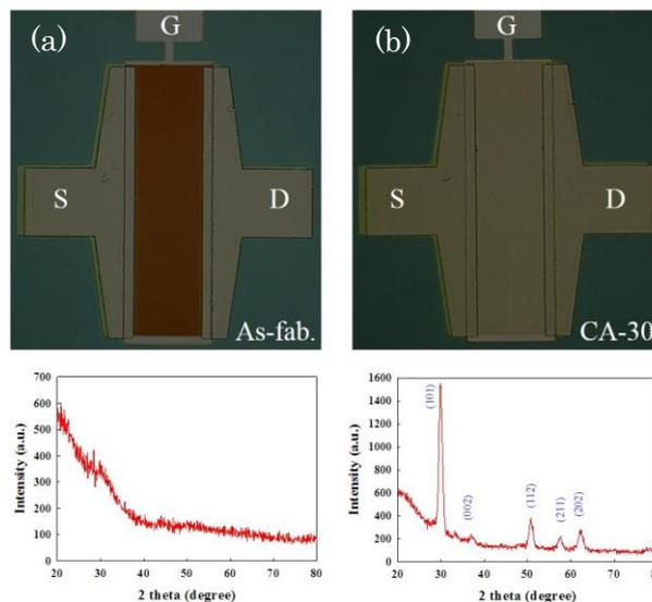
Fig. 4. OM pictures taken on a sample (a) before and (b) after going through a long annealing treatment. Corresponding XRD results are shown below, indicating that the OM images can serve as a quick check for the crystallization status of the tin oxide channel film.
