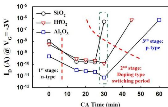
Fig. 3. Evolution of transfer characteristics with increasing CA time for TFTs having various gate dielectrics.
