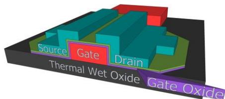
Fig. 1. The bottom-gated TFT structure employed for fabricating the test devices.
