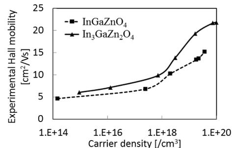
Fig. 2 Experimental Hall mobility and carrier density of In-rich IGZO thin film at room temperature. (Reference: non-In-rich InGaZnO<sub>4</sub> thin film.)
