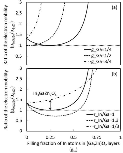
Fig. 3 Dependence of the ratio of the calculated electron mobility on the filling fraction of In atoms in In-rich IGZO thin film, with respect to (a) the filling fraction of Ga atoms and (b) the relative charge ratio.
