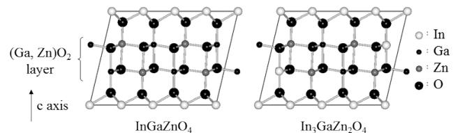
Fig. 1 Schematics of crystal structure of InGaZnO<sub>4</sub> (non-In-rich) and In<sub>3</sub>GaZn<sub>2</sub>O<sub>4</sub> (In-rich).
