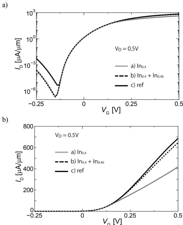
Fig. 4 Simulated I-V characteristic when composition of drain was changed. a) Log-scale plot and b) linear-scale plot. Reference is I-V curve in Fig.2 at the doping concentration of  $8 \times 10^{18} \text{ cm}^{-3}$ .
