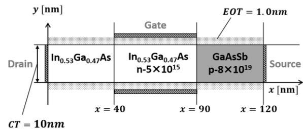
Fig. 1 Simulation structure of the tunnel FET for doping concentration dependence.
