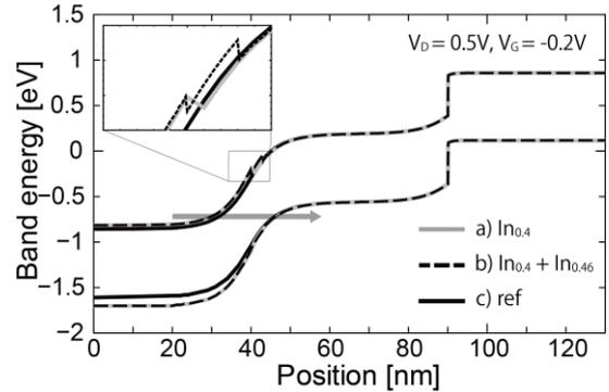
Fig. 5 Calculated band profile of the tunnel FET for composition dependence.
