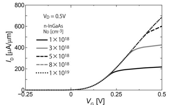
Fig. 2 Simulated I-V characteristic for different doping concentration of drain. a) Log-scale plot and b) linear-scale plot.
