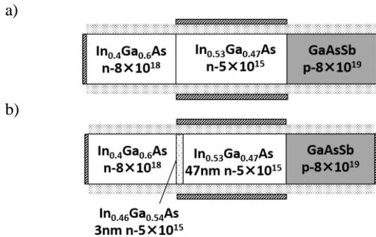
Fig. 3 Simulation structure of the tunnel FET for composition dependence. a) Abrupt junction. b) With step-graded layer.
