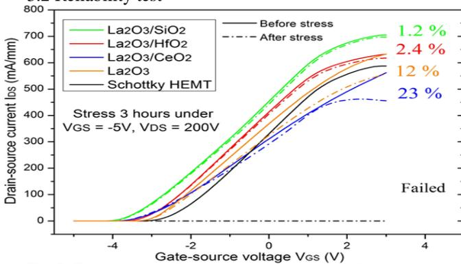
Fig.3 Comparison of current degradation and proportion after high voltage stress.
