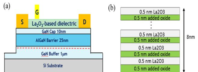
Fig.1 Schematic diagram of the (a) AlGaIn/GaN MOS-HEMT (b) nano-laminate of  $\text{La}_2\text{O}_3$ -based gate dielectric
