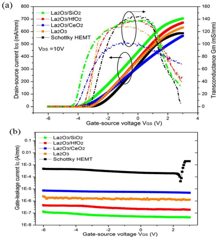
Fig.2 (a) dc transconductance, (b)  $I_G$ - $V_G$  characteristics of the studied devices.
