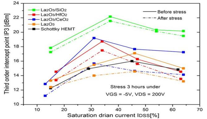
Fig.4 IP3 versus  $I_{DS}$  curves for studied device, the test frequency is 2GHz and  $V_{DS}=20V$
