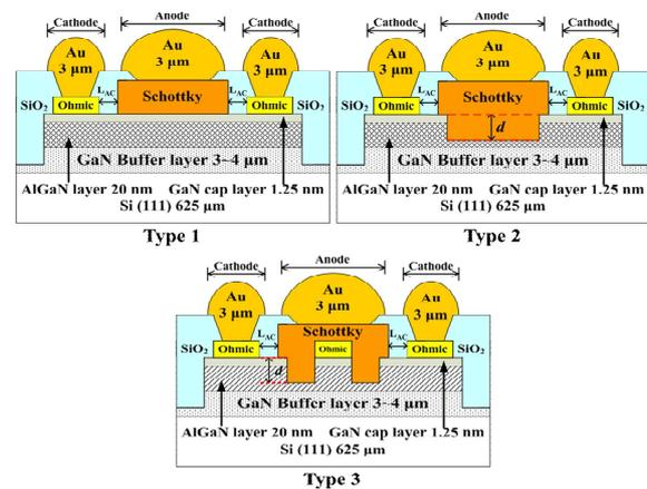
Fig. 1 The fabricated SBD structure (Type 1 = conventional SBD, Type 2 = recessed SBD, Type 3 = recessed dual anode SBD)
