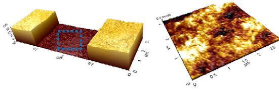
Fig. 2 AFM image of recessed region (left), rms roughness of recessed surface (right)
