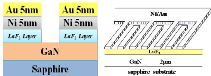
Fig. 1 The schematic structure of GaN MIS PDs with a LaF<sub>3</sub> insulating layer.
