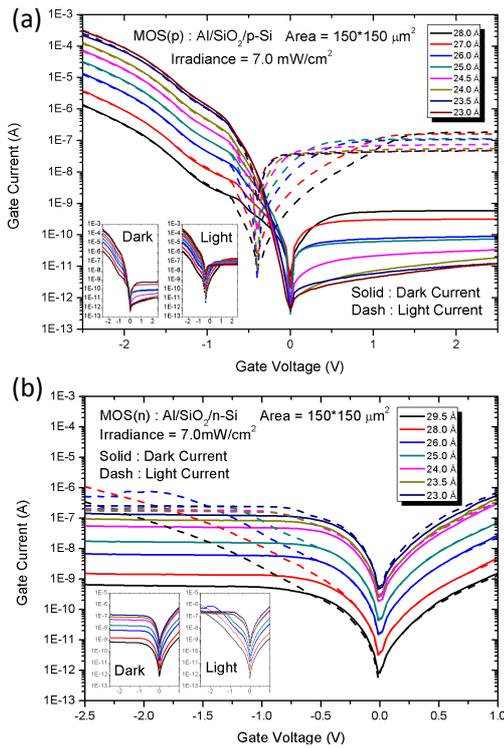
Fig. 1 Complete  $I$ - $V$  curves for dark and light current at a light intensity of  $7 \text{ mW/cm}^2$  of (a) MOS(p) with eight oxide thicknesses and (b) MOS(n) with seven oxide thicknesses.
