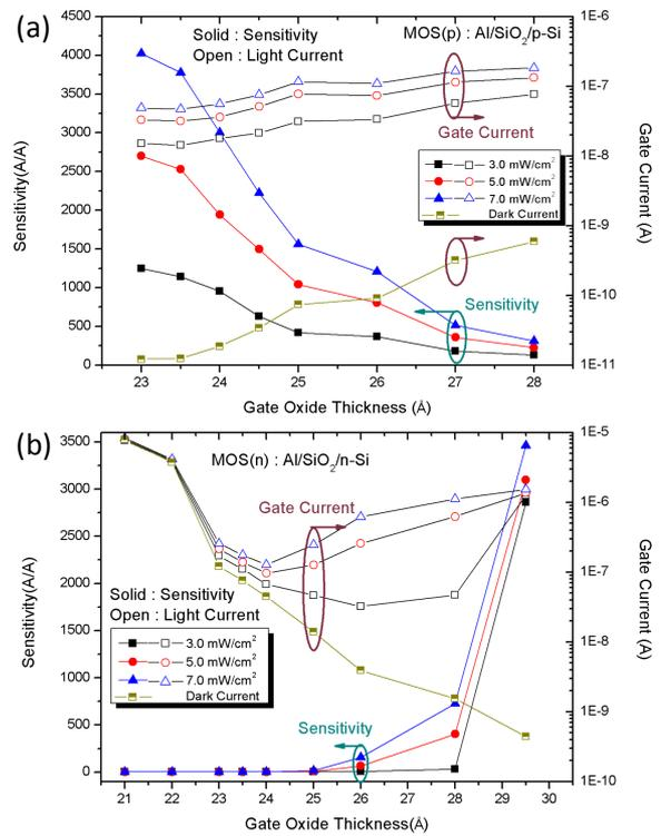
Fig. 2 Sensitivity and gate current versus oxide thickness curves of (a) MOS(p) and (b) MOS(n) at light intensities of 3, 5, and  $7 \text{ mW/cm}^2$ .
