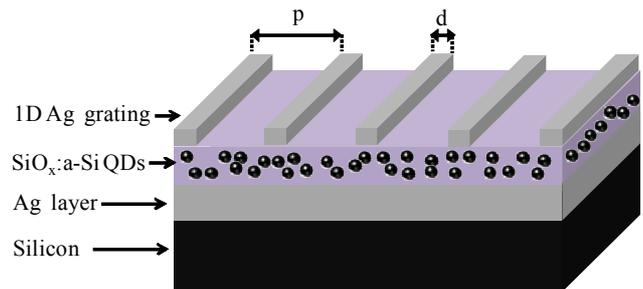
Fig. 1. The device structure of a-Si QDs LEDs with tri-layer Ag/SiO<sub>x</sub>:a-Si QDs/Ag nanostructures.
