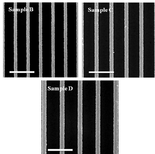
Fig. 2. The top-view SEM images of the 1D Ag grating for samples B, C, and D. Scale bar is 500 nm.
