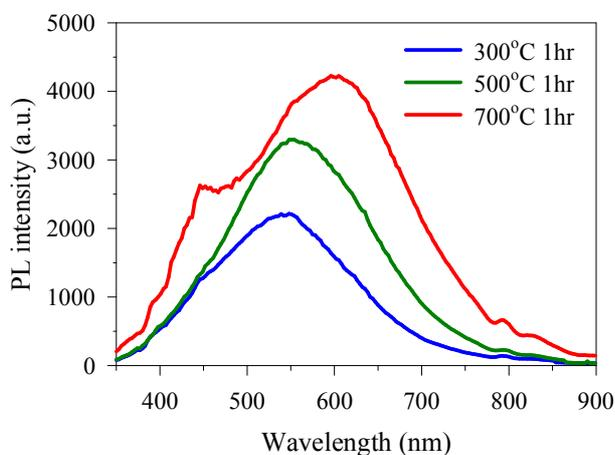
Fig. 4. The PL spectra of  $\text{SiO}_x$ :a-Si QDs films with different annealing temperatures.
