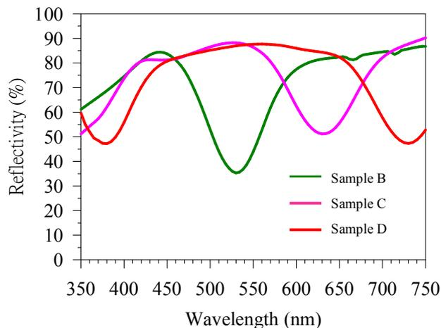
Fig. 5. The measured reflection spectra of the samples B, C, and D.
