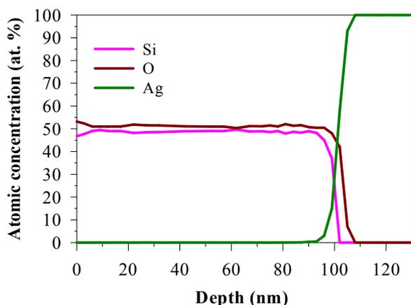
Fig. 3. The concentration-depth profiles of Si, O, and Ag atoms for  $\text{SiO}_x$ :a-Si QDs film, and at  $\text{SiO}_x$ :a-Si QDs/Ag film interface by XPS analysis.
