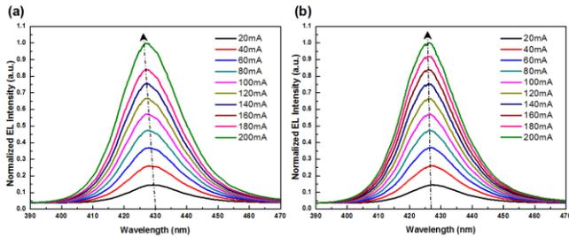
Fig. 2 Blue shifts phenomenon of the InGaN-based LEDs having the (a) CSS and (b) MOPSS.
