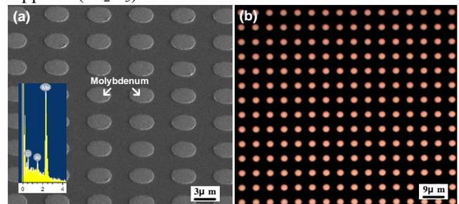
Fig. 1 (a) Scanning electron microscopy (SEM) and energy-dispersive X-ray spectroscopy (EDS or EDX) analysis, and (b) optical microscope (OM) analysis for MOPSS.
