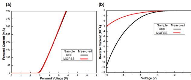
Fig. 3 (a) Forward I-V characteristics and (b) reversed I-V characteristics, of InGaN-based LEDs having the CSS and MOPSS.
