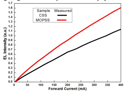
Fig. 4 EL characteristics of InGaN-based LEDs having the CSS and MOPSS.
