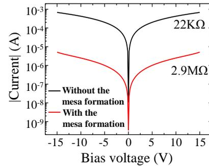
Fig. 3 I-V characteristics of the dark current before and after mesa formation
