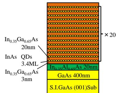
Fig. 1 Schematic drawing of stacking structure of InAs QDs layers embedded in strain-relaxation  $\text{In}_{0.35}\text{Ga}_{0.65}\text{As}$  barriers.
