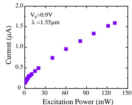
Fig. 5 Excitation power dependence of current with bias voltage of 0.9V
