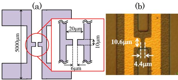
Fig. 2 (a) Schematic drawing of a dipole antenna pattern (b) zoom up of the center of antenna with mesa formation
