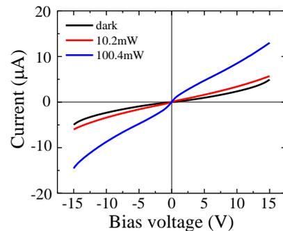
Fig. 4 I-V characteristics for the dark and excited conditions after mesa formation
