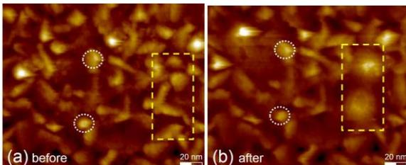
Fig. 3 AFM topographs of (2-1-4) SL before (a) and after (b) the WRITE process at +3.2 V. Dashed boxes outlined modified areas. Dotted circles indicate similar grains in (a) and (b).
