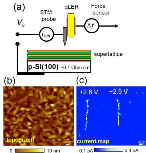
Fig. 1 (a) MSPM measurement setup. (b,c) AFM topograph and corresponding current map at a READ voltage of +1.2V after writing 2 lines for the (2-1-4) film. Numbers indicate  $V_{WRITE}$ .
