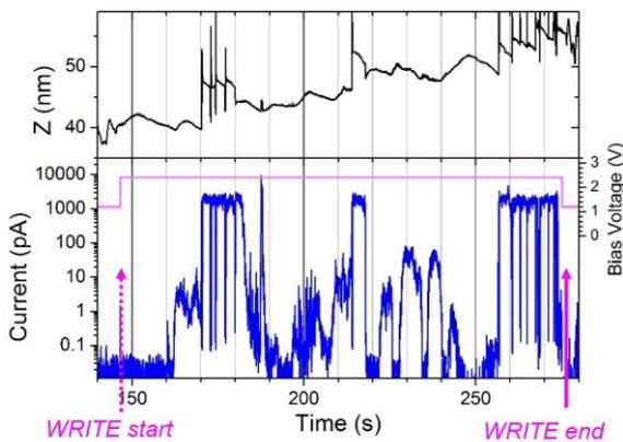
Fig. 2 STM probe position (black, top) and WRITE current (blue, bottom) at WRITE voltage (pink) for the left line in Fig.1(c).
