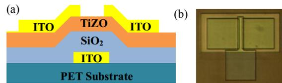
Fig. 1 (a) Schematic Cross-sectional view and (b) Micrograph of TiZO TFTs ( $W/L=100\mu\text{m}/10\mu\text{m}$ )
