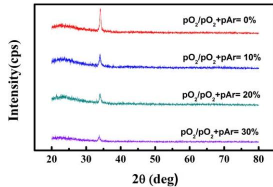
Fig.3 XRD pattern images of TiZO film deposited at various oxygen partial pressure.
