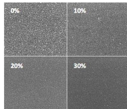
Fig.4 SEM images of TiZO TFTs deposited at various oxygen partial pressure.
