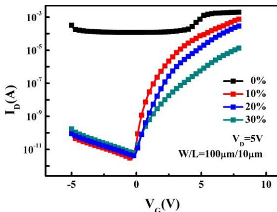
Fig.2 Transfer characteristics of TiZO TFTs fabricated at various oxygen partial pressure.
