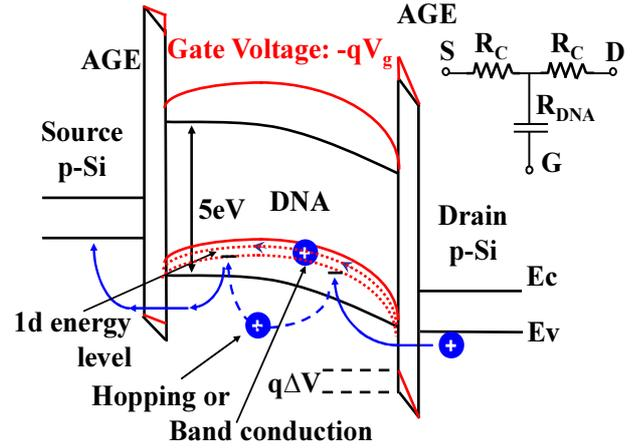
Fig. 4 Potential diagram at non-gate voltage application and at  $-qV_g$ (red line) and the equivalent circuit of DNA/Si-MOSFET.
