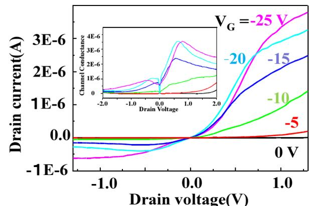
Fig.2  $I_d$ - $V_d$  characteristics of the DNA/Si-MOSFET at  $V_g$  of 0 to -25V and at room temperature. Inset is the channel conductance.
