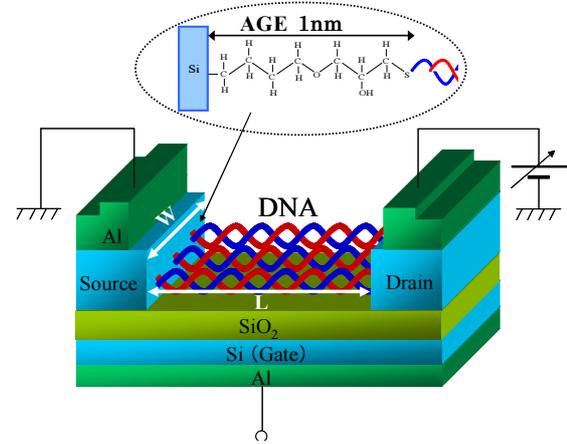
Fig.1 Schematic configuration of the DNA transistor. A 350-nm-thick p-type SOI with a resistivity of 40-60 $\Omega$ cm was used. The SOI film was thinned to 60 nm and the source/drain electrodes were left by the dry process. The inset shows the connection area of Si electrodes and the DNA molecule. An epoxy function was attached through hydrosilylation of AGE on the Si surface of the source/drain electrodes [9].
