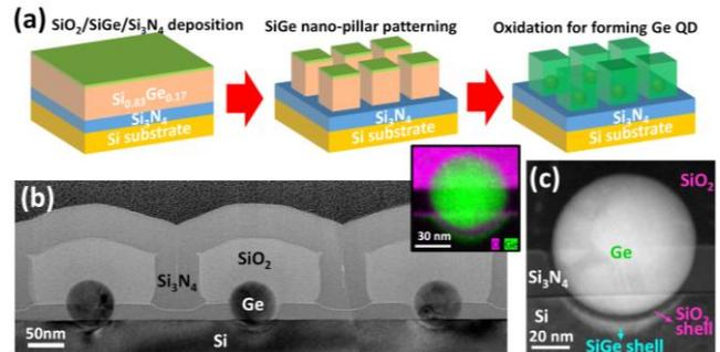
Fig. 1 I-MOS Ge NP/SiO<sub>2</sub>/SiGe-shell heterostructure. (a) Schematic of experimental fabrication procedure. (b) CTEM and EDX mapping micrographs, (c) STEM of i-MOS structure over Si substrate.
