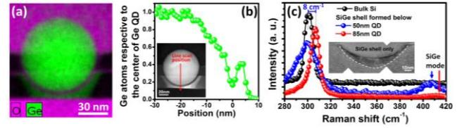
Fig. 3 (a)/(b) EDX mapping and line scan of i-MOS structure. (c) Raman spectra of SiGe shells formed right below 50 and 80nm Ge NPs and bulk Ge. The inset shows the CTEM image of a SiGe shell formed below an 85nm Ge NP that were removed by an HF dip.
