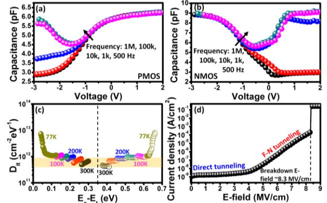
Fig. 4 (a) and (b) Frequency-dependent *C-V* characteristics of NiGe gate/SiO<sub>2</sub>/SiGe *p*-MOS and *n*-MOS capacitors. (c) Extracted *D<sub>it</sub>* (*T* = 300–77 K) and (d) *I-V* characteristic of NiGe/SiO<sub>2</sub>/SiGe capacitors.
