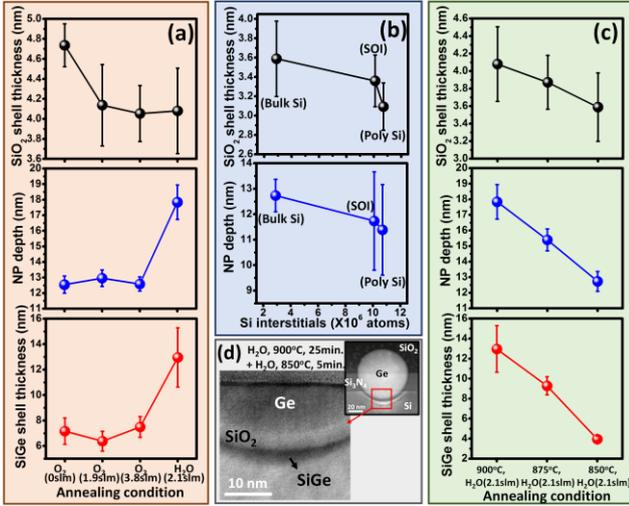
Fig. 2 Thickness of interfacial SiO<sub>2</sub> layer and SiGe shell as well as depth of penetration for Ge NP are tunable by flow-rates of (a) annealing gas, (b) Si interstitials flux, and (c) temperature. (d) CTEM images for 65nm Ge NPs formed by *in situ* post-oxidation annealing in an H<sub>2</sub>O ambient at 850°C.
