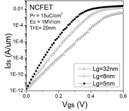
**Fig. 5.** Id-Vg curves of NCFETs with  $L_g=16, 5$  and  $3\text{nm}$ .
