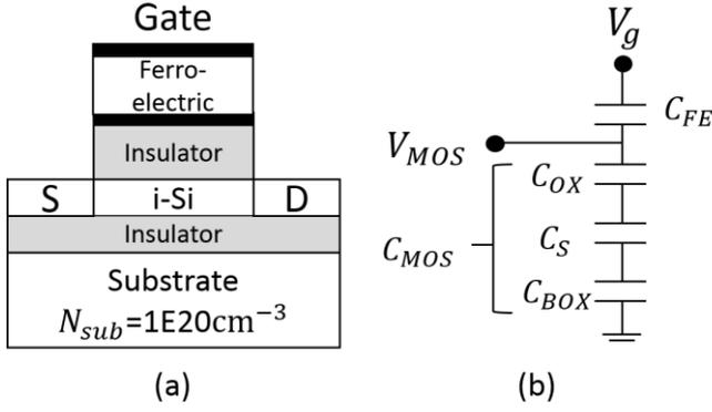
**Fig. 1.** (a) Schematic sketch of the UTB NCFET [3,4]. (b) Capacitance model of the NCFET.
