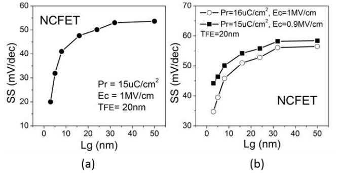
**Fig. 6.** Improved SS with decreasing  $L_g$  for NCFETs with different ferroelectric materials.
