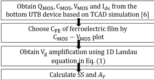
**Fig. 2.** Numerical simulation flow of NCFET in this work.  $Q_{MOS}$  is the gate charge of the UTB device.
