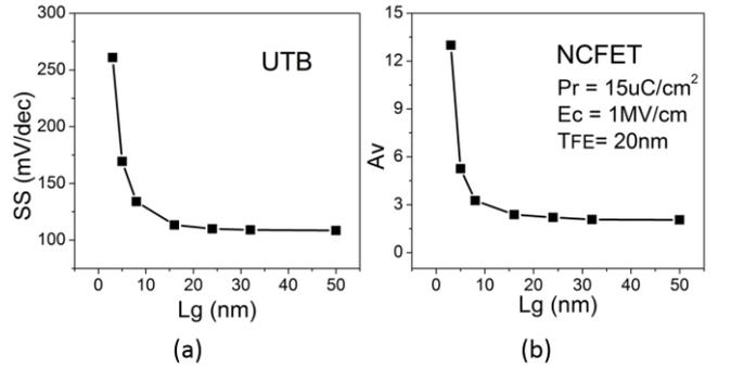
**Fig. 7.** (a) SS versus  $L_g$  for the bottom UTB MOSFET. (b)  $A_V$  versus  $L_g$  for the NCFET. The  $A_V$  is calculated by Eq. (4a).
