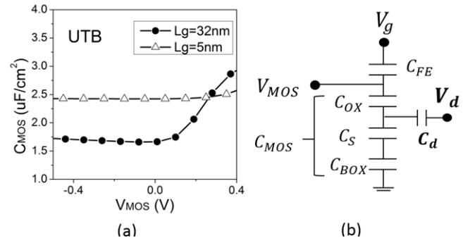
**Fig. 8.** (a) Comparison of the CV curves for the bottom UTB MOSFETs with  $L_g=32\text{nm}$  and  $5\text{nm}$ . (b) Capacitance model of the short-channel NCFET considering drain coupling.
