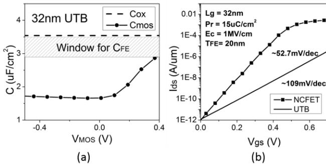
**Fig. 4.** (a) CV curve of the bottom UTB MOSFET. (b) Id-Vg curves of the NCFET and UTB device with  $L_g=32\text{nm}$ .
