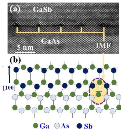
Fig. 1. (a) HRTEM image showing the periodic 2-D IMF array at the GaSb/GaAs interface. IMFs allow the relaxation of majority of the strain resulting from the lattice mismatch. (b) Schematic illustration of the misfits at the GaSb/GaAs interface.
