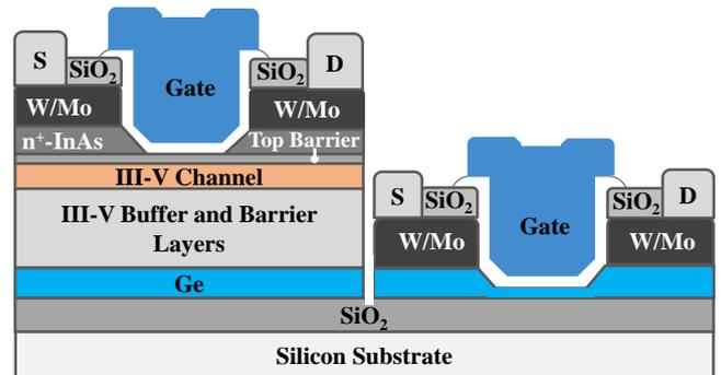
Fig. 2. Schematic of the first demonstration of InAs n-FETs and Ge p-FETs monolithically integrated on a Si substrate. The thickness of the III-V buffers is less than 120 nm.
