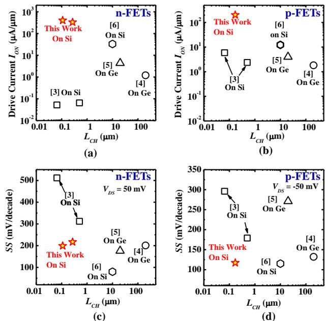
Fig. 3. (a)  $I_{ON}$  vs.  $L_{CH}$  for  $In_{1-x}Ga_xAs$  n-FETs, (b)  $I_{ON}$  vs.  $L_{CH}$  for  $Si_{1-x}Ge_x$  p-FETs [ $|V_{GS}-V_{TH}|=1$  V and  $|V_{DS}|=1$  V, except in [3] where  $|V_{DS}|=0.5$  V], (c)  $SS$  vs.  $L_{CH}$  for  $In_{1-x}Ga_xAs$  n-FETs, and (d)  $SS$  vs.  $L_{CH}$  for  $Si_{1-x}Ge_x$  p-FETs. Note that the comparison is made among co-integrated SiGe p-FETs and InGaAs n-FETs on the Si substrate.
