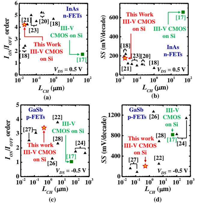
Fig. 5. Benchmark plot comparing (a)  $I_{ON}/I_{OFF}$  ratio of InAs n-FETs, (b)  $SS$  of InAs n-FETs, (c)  $I_{ON}/I_{OFF}$  ratio of GaSb p-FETs, and (d)  $SS$  of GaSb p-FETs. Our work achieved the best value of  $I_{ON}/I_{OFF}$  ratio and  $SS$  for III-V CMOS integrated on the Si substrate.
