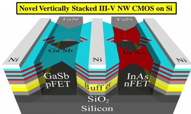
Fig. 4. 3D schematic of the vertically-stacked III-V nanowire CMOS on a common Si platform. This was enabled by growth of alternating layers of GaSb (p-FET channel) and InAs (n-FET channel) on a III-V buffer grown by IMF technique on a GeOI substrate (from Fig. 1 of Ref. 1).
