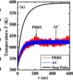
Fig. 6 Channel  $T$ - $t$  plot shows high  $f$  AC and PRBS signal result much lower channel  $T$  than DC signal.
