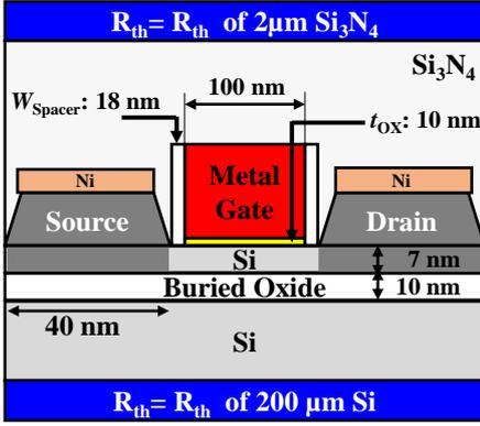
Fig. 1 Schematics of the SOI MOSFET for modeling and measurement. The dimensions used for simulation were indicated in the schematics. The Ni layer thickness is 20 nm, the raised S/D height is 11 nm and the gate height is 95 nm.
