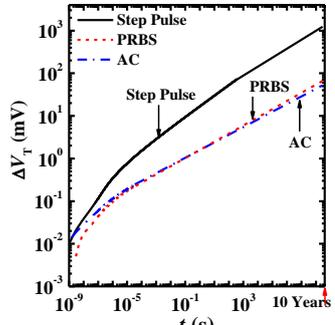
Fig. 8  $\Delta V_T$ - $t$  plot is extended to 10 years. PRBS stress signal shows slightly higher  $\Delta V_T$ .
