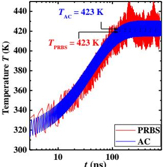
Fig. 7 PRBS and AC signals at the same bit rate show similar channel  $T$  profiles.
