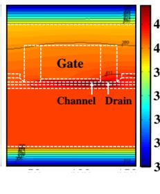
Fig. 5 Transient temperature profile in the device channel high  $f$  AC and PRBS signal region shows the highest  $T$  of 430 K.
