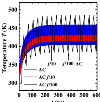
Fig. 9 Channel  $T$ - $t$  plot shows higher  $f$  AC results in lower base channel  $T$  and smaller oscillation amplitude.
