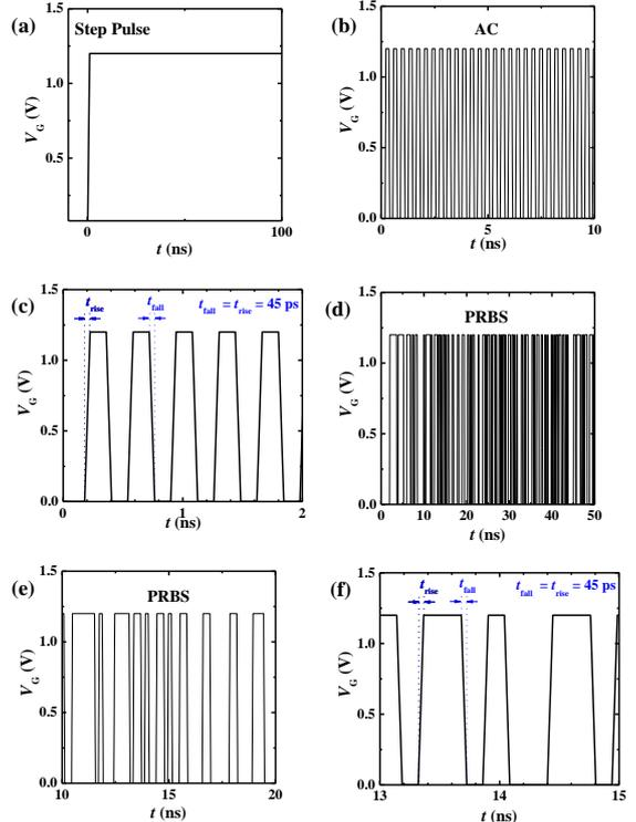
Fig. 3 (a), (b), (d) are the DC, AC and PRBS gate signals used for channel temperature and  $V_T$  shift calculation. The amplitude of the signals are 1.2 V. (c) is the zoomed-in AC signal within 2 ns. (e) and (f) are the zoomed-in PRBS signals with 10 and 2 ns, respectively. The rise and fall time for the AC and PRBS signals are both 45 ps. The minimum time interval for  $V_G = 1.2$  V in the PRBS is 90 ps and that for the AC signal is also 90 ps.
