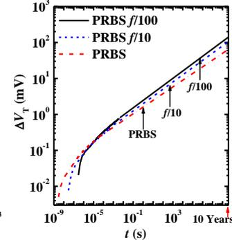
Fig. 12  $\Delta V_T$ - $t$  plot are extended to 10 years for various  $f$  circuit speed, lower  $f$  PRBS signals lead to much higher  $\Delta V_T$ .
