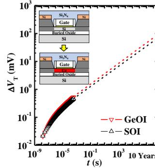
Fig. 13  $\Delta V_T$ - $t$  plot are extended to 10 years for SOI and GeOI substrates.
