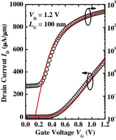
Fig. 4  $I_D$ - $V_G$  characteristics by simulation (solid) and by measurement (dot) match well.
