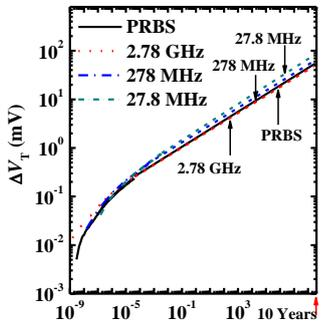
Fig. 10  $\Delta V_T$ - $t$  plot is extended to 10 years for various  $f$  AC stress signal, lower  $f$  AC signals lead to much higher  $\Delta V_T$ .
