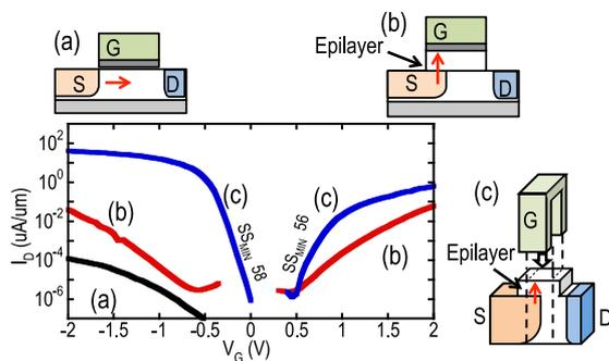
Fig. 4 Typical transfer characteristics of three TFET architectures: (a) conventional lateral type ( $V_D = |1|$  V,  $L_G = 1$   $\mu$ m), (b) parallel-plate type ( $V_G = |1|$  V,  $L_G = 500$  nm), and (c) FinFET-like TFETs ( $V_D = |0.2|$  V,  $L_G = 100$  nm). For conventional TFET, only p-type  $I_D$ - $V_G$  is plotted.
