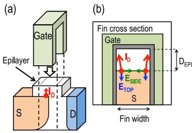
Fig. 1 Schematics of tunnel FinFET featuring ultrathin epitaxial channel inserted between gate and source, in the present study. Inset shows channel cross-section of tunnel FinFET, indicating synthetic electric field at the source/epichannel interface.
