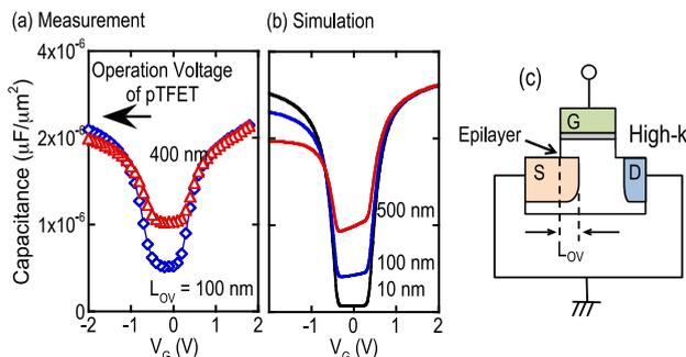
Fig. 9 Typical C-V characteristics of pTFET featuring ultrathin epitaxial channel. Variations in source-gate overlapped length ( $L_{ov}$ ) exist. (a) Experimental and (b) simulation results. (c) Measurement setup.
