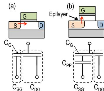
Fig. 10 Schematic capacitance distribution models for (a) conventional and (b) epitaxial channel TFETs. Distribution of source and drain capacitances are also indicated. In the case of (b), parallel-plate capacitor is inserted.
