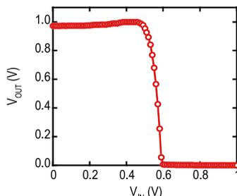
Fig. 6 Typical  $V_{IN}$ - $V_{OUT}$  characteristics of tunnel FinFET CMOS inverter.  $L_G = 1$   $\mu$ m.  $V_{DD} = 1$  V.
