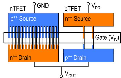
Fig. 5 Device configuration in tunnel FinFET CMOS inverter.  $V_{IN}$  is added for gate electrode. Numbers of fin channels are 2 and 18 for p- and n-type tunnel FinFETs, respectively.
