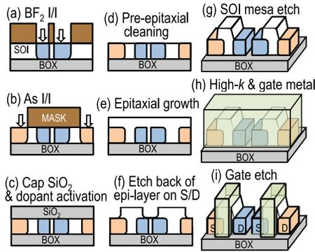
Fig. 2 Process flow of CMOS tunnel FinFETs.
