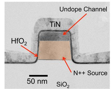
Fig. 3 Typical XTEM image of tunnel FinFET (p-type) channel.
