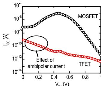
Fig. 7 Comparison of short-circuit current of MOSFET and tunnel FinFET CMOS inverters.  $L_G$  of TFETs and MOSFETs are 1 and 8  $\mu$ m, respectively.  $V_{DD} = 1$  V for both inverters.
