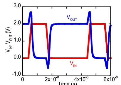
Fig. 8 Simulation of Si CMOS TFET inverter.  $V_{IN} = 2$  V. Conventional type Si TFET is simulated [7].
