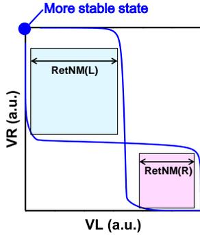
Fig.1. Example of butterfly curves in the retention condition (RetNM definition is shown). The more stable state is corresponding to the larger opening eye of the butterfly curves.
