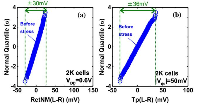
Fig.5. (a) Retention noise margin mismatch (RetNM(L-R)) at  $V_{DD}=0.6\text{V}$  and (b) pFET  $|V_{TH}|$  mismatch (Tp(L-R)) distributions.
