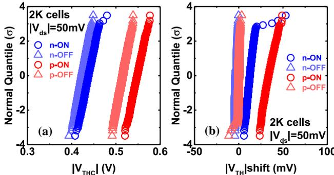
Fig.6. (a)  $|V_{THC}|$  and (b)  $|V_{TH}|$  shift distributions after applying stress.
