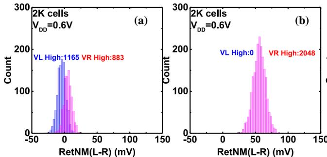
Fig.8. Histograms of RetNM(L-R) for both VR(High) and VL(High) bits at power-up (a) before and (b) after applying stress.
