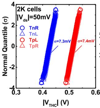
Fig.3. Measured  $|V_{THC}|$  distributions of the pFETs and nFETs at  $|V_{ds}|=50\text{mV}$ .
