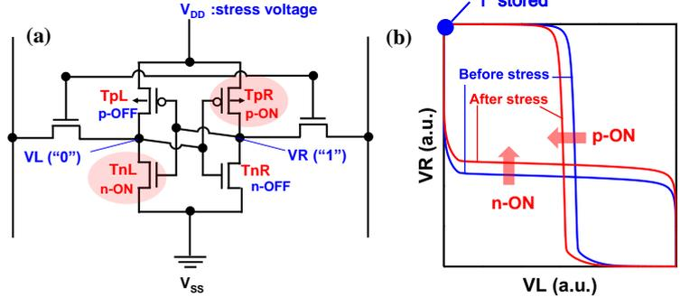
Fig.2. (a) A schematic of 6T-SRAM cell. (b) Butterfly curves before and after stress. In this example, it is assumed that VL is low and VR is high. The right pFET is p-ON and the left nFET is n-ON.
