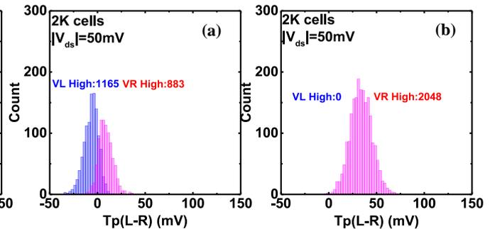
Fig.9. Histograms of Tp(L-R) for both VR(High) and VL(High) bits at power-up (a) before and (b) after applying stress.
