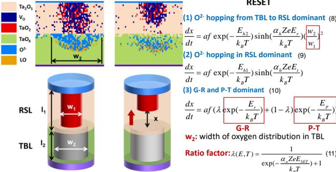
Fig. 3 RESET process is modeled based on the simulated CF evolution. The increase of gap distance ( $x$ ) is determined by processes (1)~(3).
