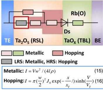
Fig. 5 Equivalent circuit of conduction.
