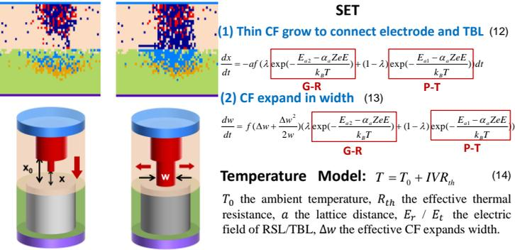
Fig. 4 SET process is modeled based on the simulated CF revolution and is decided by gap distance ( $x$ ) and CF width ( $w$ ).
