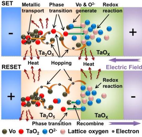
Fig. 1 Schematic physical processes in bi-layered TaO<sub>x</sub>-RRAM.
