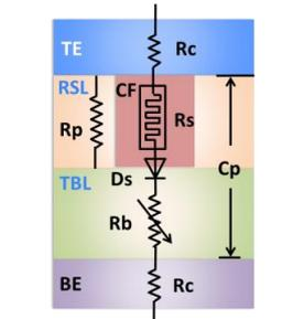
Fig. 12 Equivalent circuit with parasitic effects.
