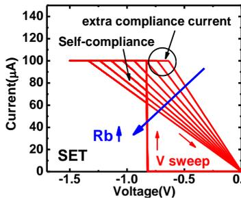
Fig. 11 The increase of TBL resistance leads to obvious self-compliance.
