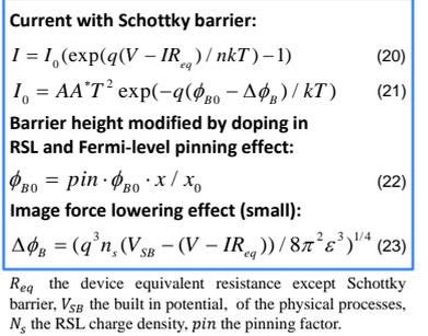
Fig. 7 The Schottky barrier model between RSL/TBL.
