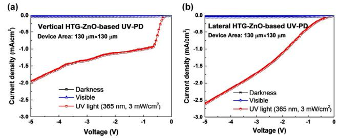
Fig. 5. Comparisons of experimental J-V characteristics of vertical and lateral HTG-ZnO-based UV-PDs irradiated by visible and UV lights.
