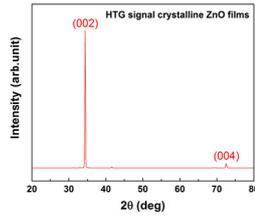
Fig 3 XRD pattern of signal crystalline HTG-ZnO films with signal crystalline structure.
