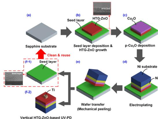
Fig. 1 The key process flow of vertical structure HTG-ZnO-based UV-PD via a mechanical peeling wafer transfer technique.
