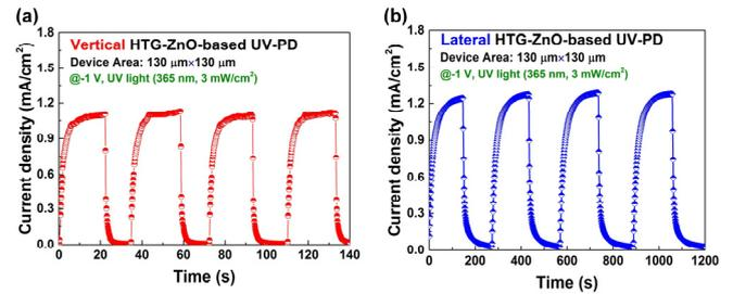
Fig. 6. Transient response of photocurrent density of (a) vertical and (b) lateral HTG-ZnO UV PDs. Wavelength and intensity of UV light are 365 nm and 3 mW/cm<sup>2</sup>, respectively.
