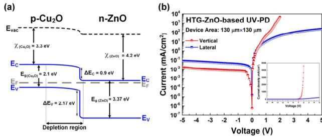
Fig. 4. (a) The energy band diagram of p-Cu<sub>2</sub>O/HTG-ZnO UV-PD under thermal equilibrium. (b) Experimental J-V characteristics of the fabricated HTG-ZnO-based UV-PDs in the dark. The inset shows the same J-V curves in linear scale.
