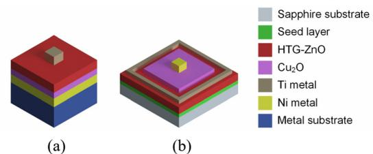
Fig. 2 Schematic diagrams of (a) vertical and (b) lateral structure HTG-ZnO UV-PD structures.
